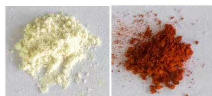
**Figure S1.** Colors of UiO-66-NH<sub>2</sub> (right) and UiO-66-NH<sub>2</sub>@Calcein (left).
