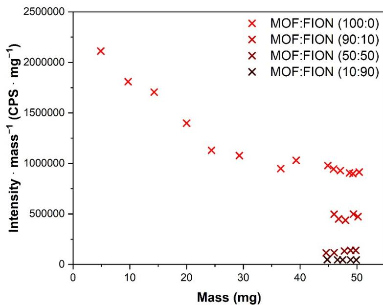
**Figure S4.** Single data points of photoluminescence quantification measurement ( $\lambda_{em} = 617$  nm).
