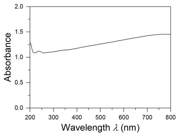
**Figure S5.** Absorption spectrum of a 2.2 wt-% dispersion of spray-dried FION.
