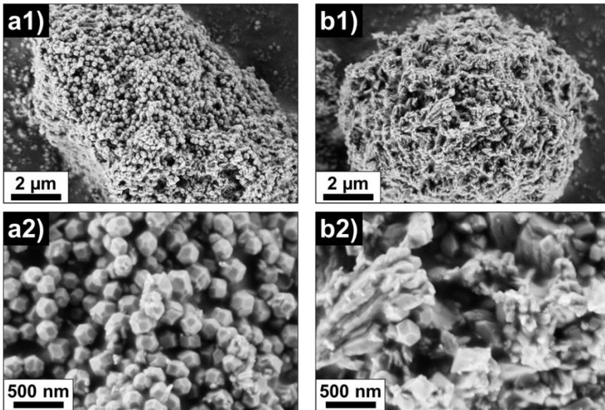
**Figure S2.** SEM of the obtained MOFFIOS products depending on the mass-related MOF:FION ratio **a 1-2)** 1:3; **b 1-2)** 3:1 (1: overview; 2: detail).
