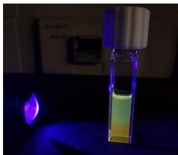
Figure S5: Photograph of a cuvette containing a BTaz-Ph-PXZ solution in chloroform after irradiation with an N_2 laser emitting at 337 nm, showing a clear colour change on the top part of the solution where the light hits the sample, whereas the bottom part retains the same colour as the pristine solution. This colour change was not, or barely, visible in toluene.
