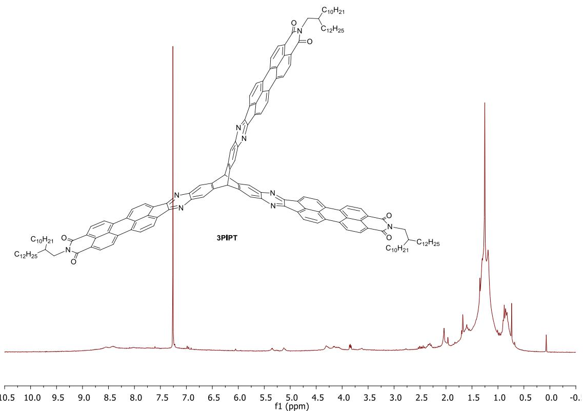
**Figure S12.**  $^1\text{H}$ -NMR spectrum of **3PIPT** in  $\text{CDCl}_3$ .
