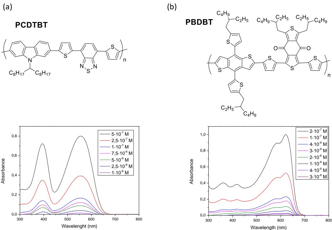
**Figure S26.** UV-Vis absorption spectra recorded in chloroform solutions for (a) **PCDTBT** and (b) **PBDBT**
