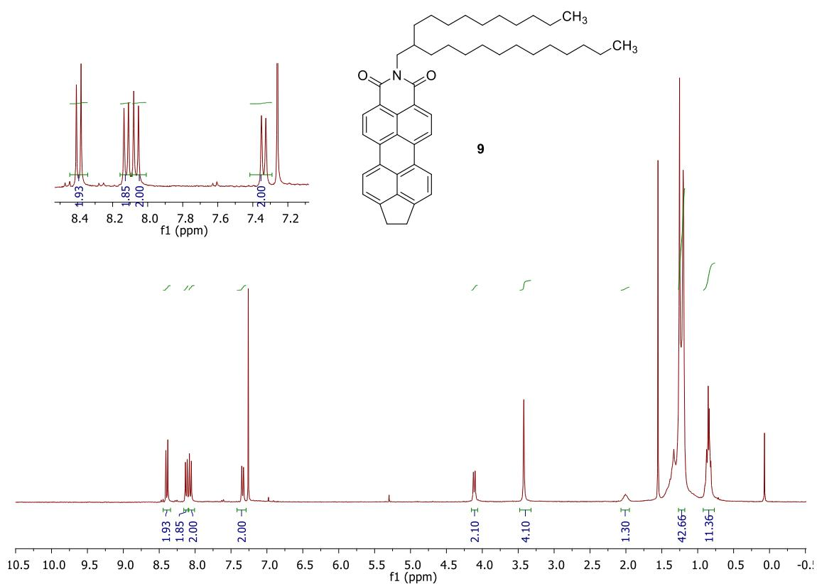
**Figure S5.** <sup>1</sup>H-NMR spectrum of **9** in CDCl<sub>3</sub>.
