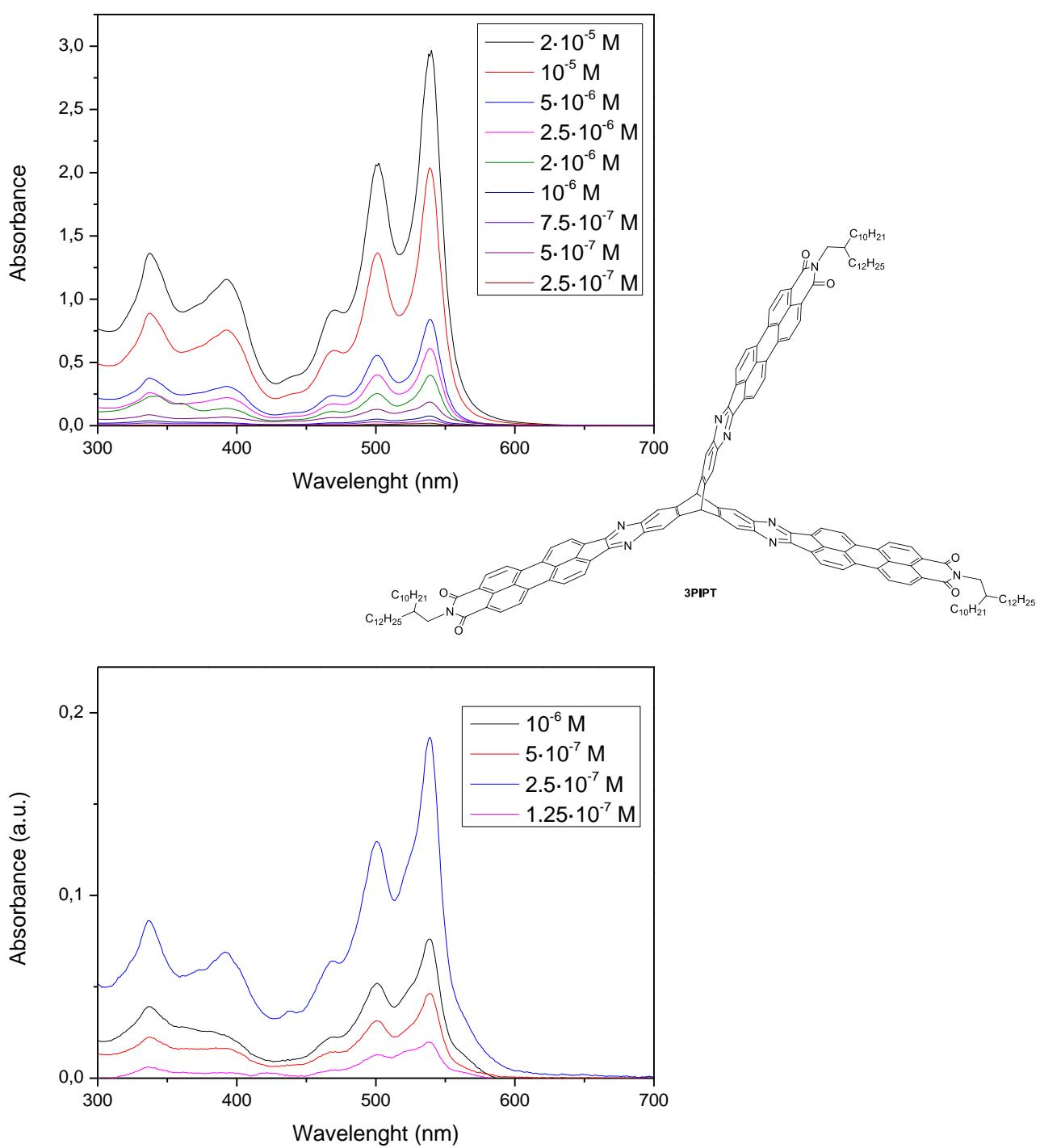
**Figure S22.** Solution UV-Vis spectra of **3PIPT** at different concentrations.
