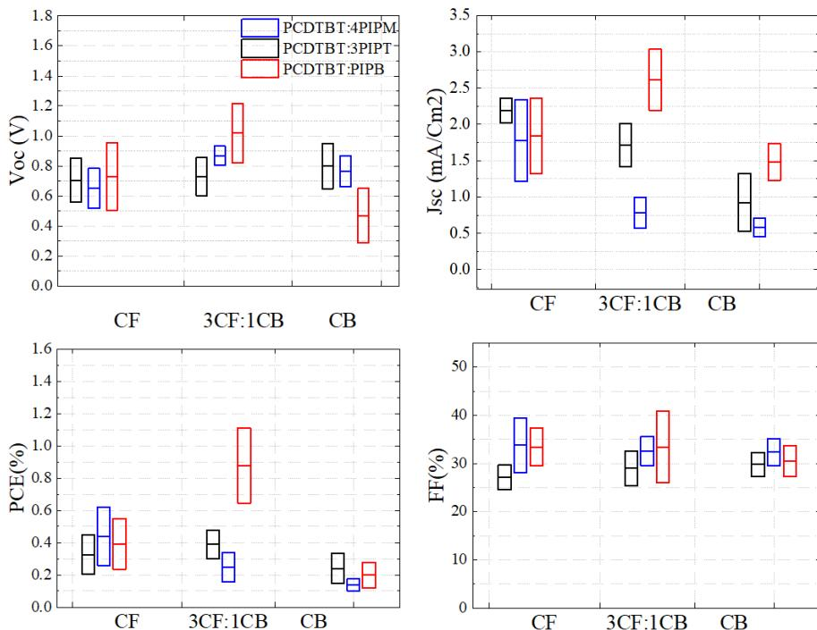
**Figure S27.** Box plot of the photovoltaic parameters of devices with different solvents for the different active layers **PCDTBT:PIPb** (red), **PCDTBT:3PIPT** (black) and **PCDTBT:4PIPM** (blue).
