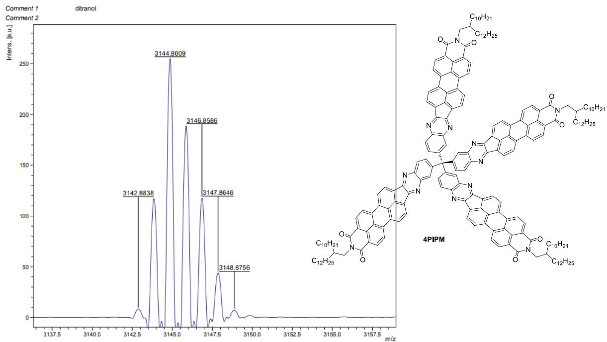
**Figure S18.** MALDI-HRMS ( $m/z$ ) mass spectrum of **4PIPm**.
