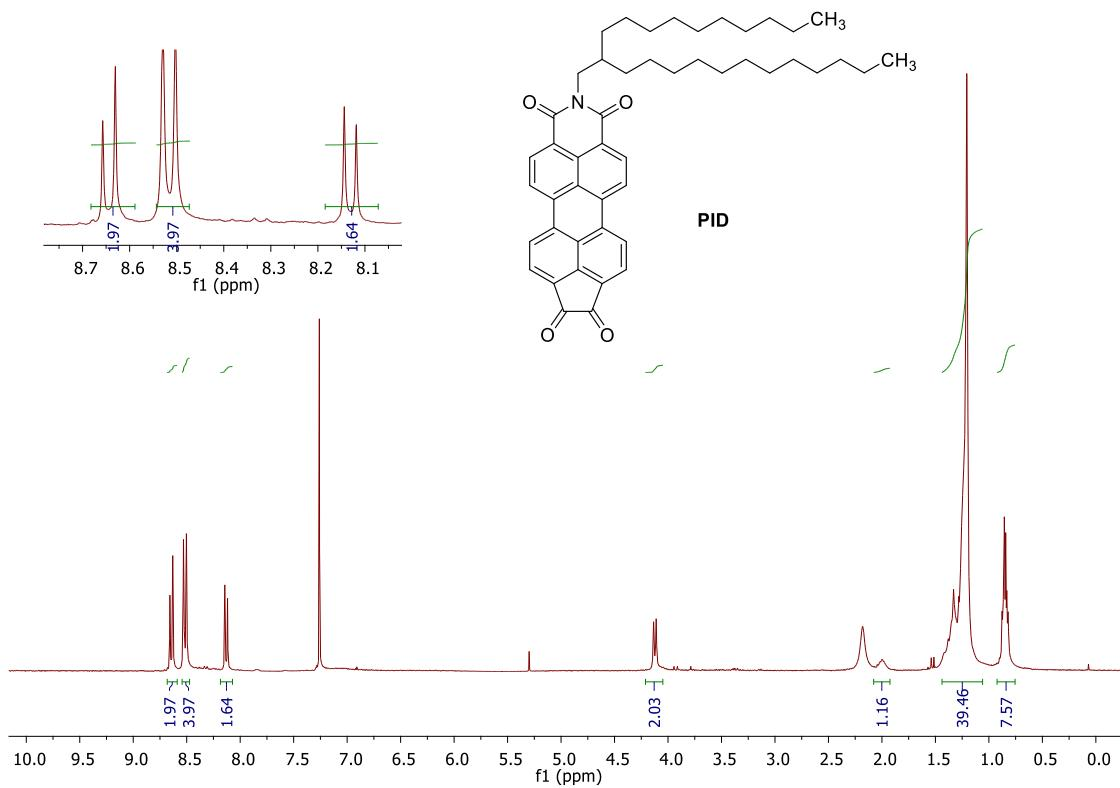
**Figure S8.**  $^1\text{H}$ -NMR spectrum of **PID** in  $\text{CDCl}_3$ .
