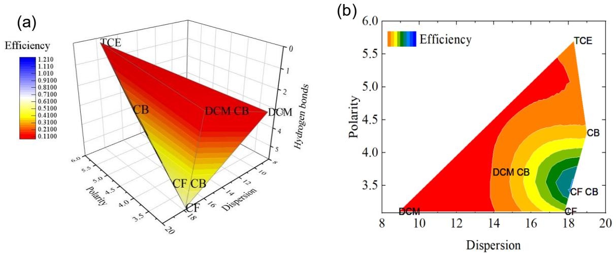
**Figure S29.** (a) Efficiency surface of photovoltaic devices on the Hansen solubility parameter space for different solvents used for the active layer formation. TCE: tetrachloroethane, DCM: dichloromethane, CB: chlorobenzene and CF: chloroform. (b) 2D projection of the efficiency surface on the polarity/dispersion axes.
