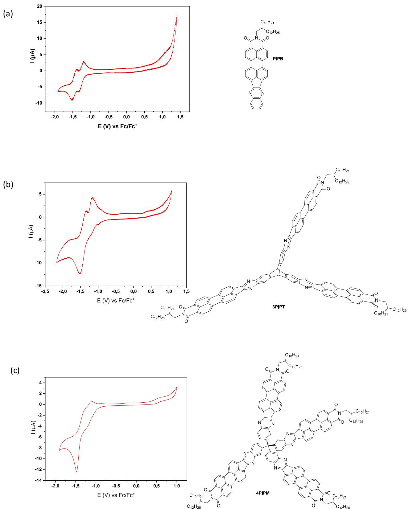
**Figure S25.** Cyclic voltammetry of (a) **PIPB** and 0.1 M TBAPF<sub>6</sub>, (b) **3PIPT** and 0.1 M TBAPF<sub>6</sub> and (c) **4PIPM** and 0.1 M TBAPF<sub>6</sub>, all of them in dichloromethane solution.
