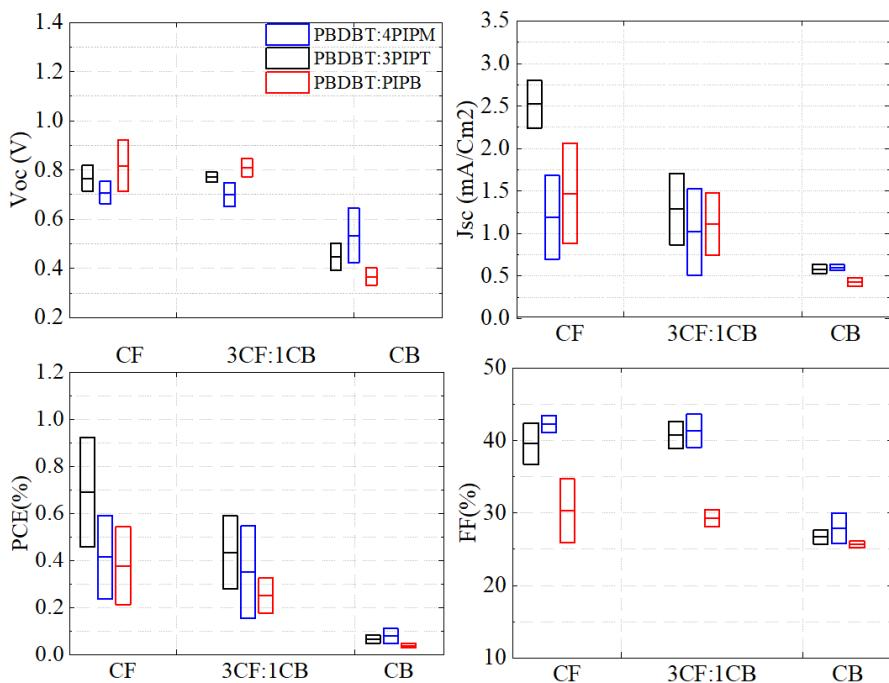
**Figure S28.** The box plot of the photovoltaic parameters of devices with different solvents for different active layers **PBDBT:PIPb** (red), **PBDBT:3PIPT** (black) and **PCDTBT:4PIPM** (blue).
