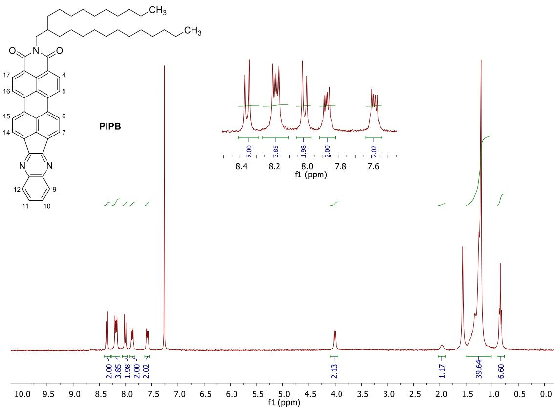
**Figure S10.** <sup>1</sup>H-NMR spectrum of **PIP<sub>B</sub>** in CDCl<sub>3</sub>.
