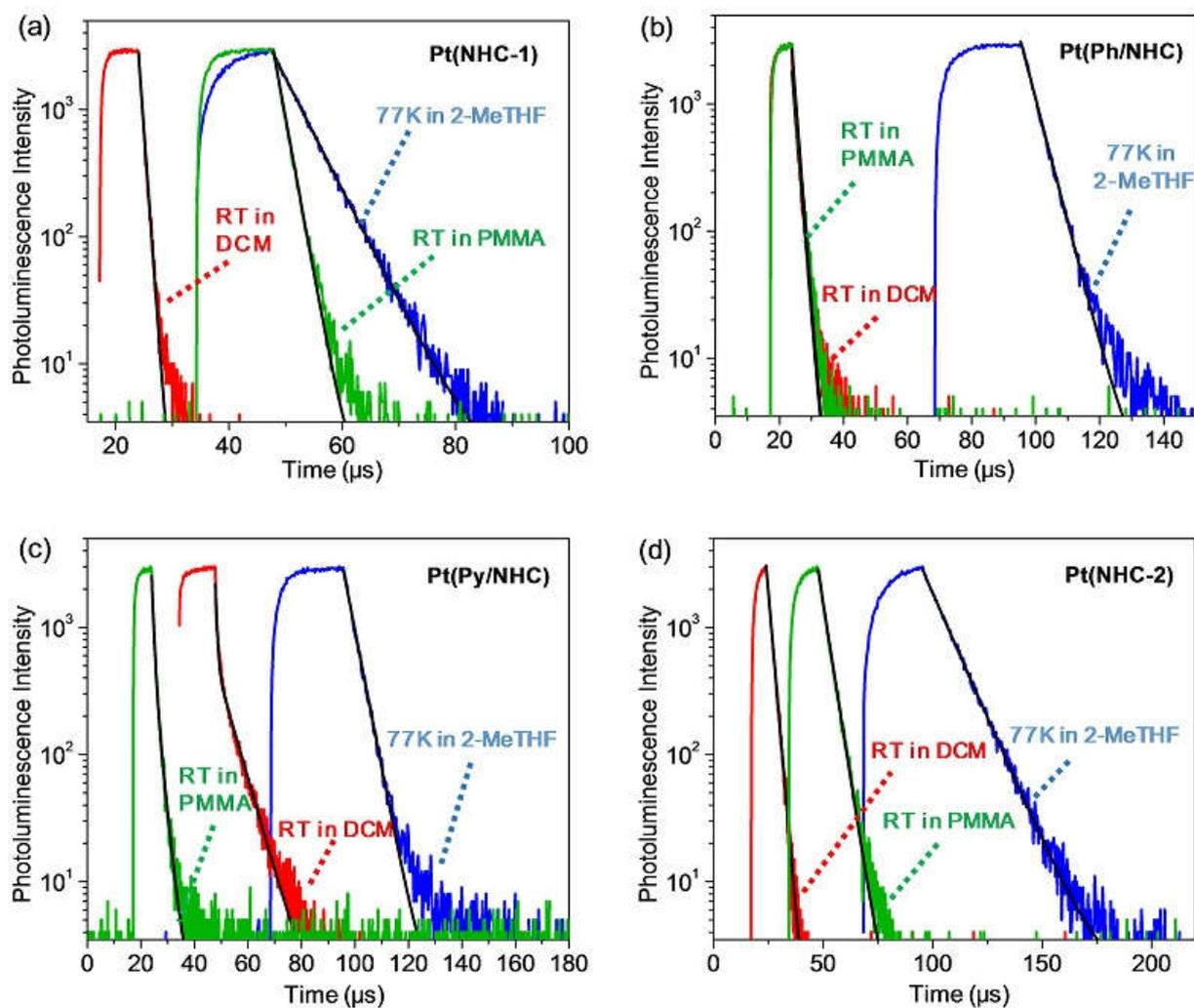
**Figure S4.** Transient decay spectra of (a) Pt(NHC-1), (b) Pt(Ph/NHC), (c) Pt(Py/NHC) and (d) Pt(NHC-2) in various conditions. The solid black lines represent biexponential fit of the experimental data.
