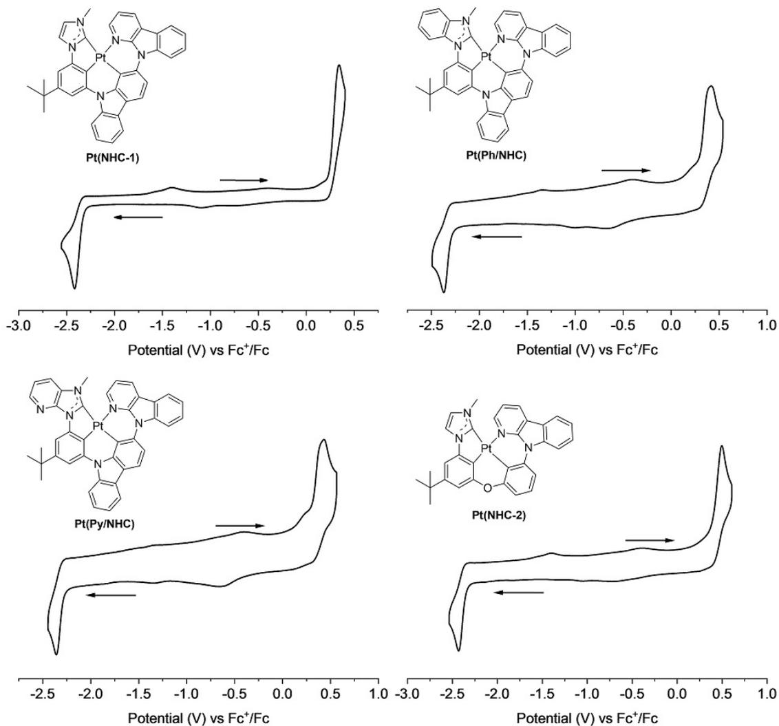
**Figure S1.** The cyclic voltammetry (CV) of tetradentate Pt(II) complexes measured in *N,N*-dimethylformamide under an nitrogen atmosphere.
