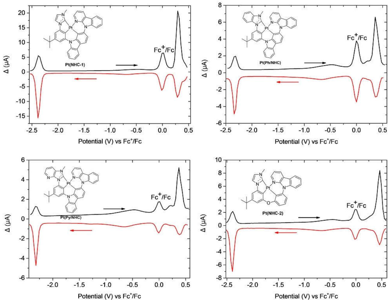
**Figure S2.** The different pulsed voltammetry (DPV) of tetradentate Pt(II) complexes measured in *N,N*-dimethylformamide under an nitrogen atmosphere.
