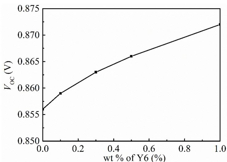
**Fig. S1**  $V_{oc}$  as a function of Y6 weight ratio in the blend films.
