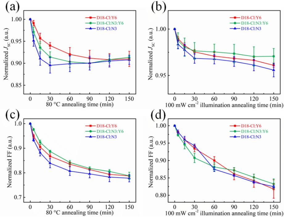
**Fig. S5** Nonencapsulated device stability statistics ( $J_{SC}$ , FF) that annealed (a,c) at 80 °C and (b,d) under AM 1.5G radiation (100 mW cm<sup>-2</sup>) in ambient atmosphere.
