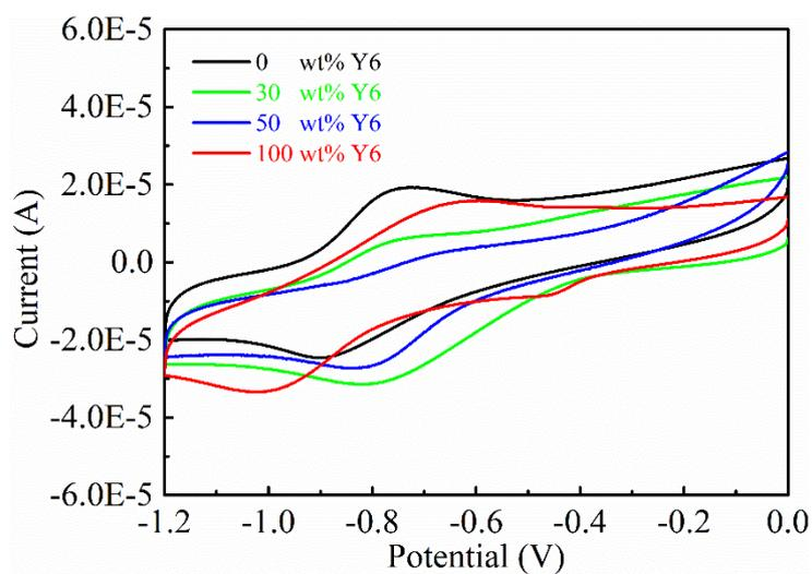
**Fig. S4** The cyclic voltammetry curves of blend films with different Y6 weight ratios.
