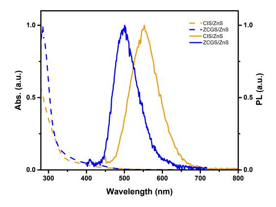
**Figure S8.** The absorption (dashed line) and emission (solid line) spectra of ZnCuGaS/ZnS core/shell quantum dots which used as a control in the experiment of PV response of LSCs as a function of the distance. As zinc was doped, the emission was blue shifted about 100 nm.
