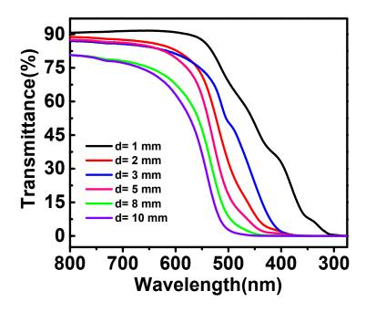
**Figure S3.** Transmittance of the synthesized  $(dMDAEMA)_2[Mo_6I_{14}]$ -PMMA hybrid with dye concentration of C=1 mg/ml at various thickness: d=1 mm (black line), d=2 mm (red line), d=3 mm (blue line), d=5 mm (pink line), d=8 mm (green line) and d=10 mm (violet line).
