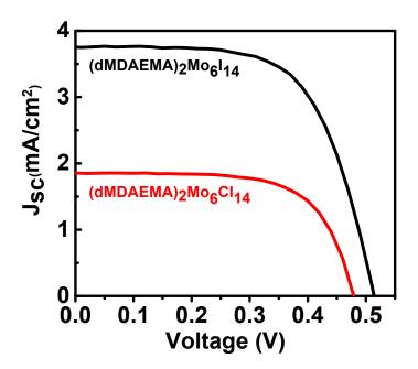
**Figure S2.** The J-V curves of LSC device at concentration C=1mg/ml and thickness of d= 3mm with different halide ligands contained dyes,  $(dMDAEMA)_2[Mo_6I_{14}]$  (black line) and  $(dMDAEMA)_2[Mo_6Cl_{14}]$  (red line).
