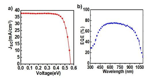
**Figure S7**. a) I-V curve of Si PV cell. The PCE of  $16.0 \pm 0.1\%$ , the short circuit current density ( $J_{SC}$ ) of  $37.8 \pm 0.1$  mAcm-2, open circuit voltage ( $V_{OC}$ ) of  $0.565 \pm 0.01$ V, and a fill factor of  $74.7 \pm 0.1$  % were observed. **b)** EQE of Si PV cell.
