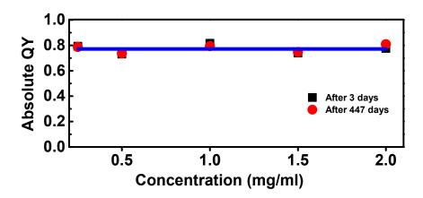
**Figure S4.** The absolute QY of the hybrid LSC plate after three days (black square) and 15 months after the fabrication (red circle) with various dye concentrations. The unchanged QY suggests that the LSC device made from the hybrid is stable against moisture and light.
