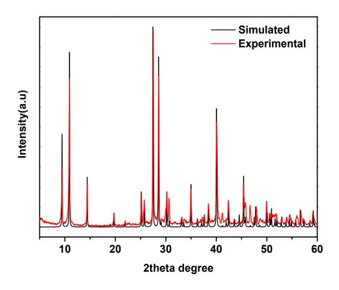
Figure S5. Comparison of experimental and simulated XRD patterns of  $Cs_2Mo_6I_{14}$ . The powder X-ray pattern of  $Cs_2Mo_6I_{14}$  perfectly matched with the calculated pattern from single crystal data.
