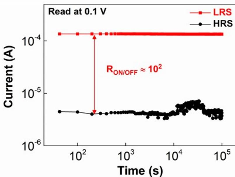
**Figure S11.** Typical retention time with read at 0.1 V during 10<sup>5</sup> s for HRS (black) and LRS (red).
