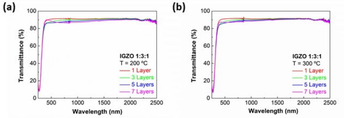
**Figure S1.** Optical transmittance of IGZO thin films with different thickness annealed at (a) 200 °C and (b) 300 °C.
