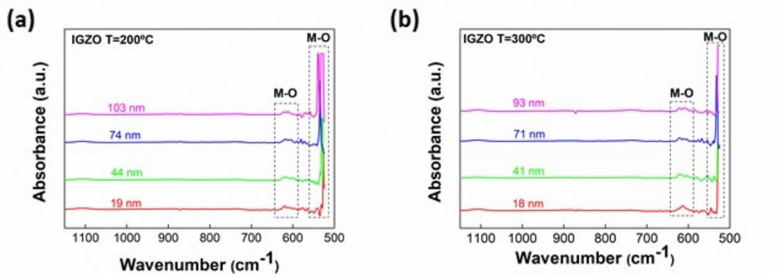
**Figure S2.** FTIR spectra of IGZO thin films with different thickness annealed at (a) 200 °C and (b) 300 °C.
