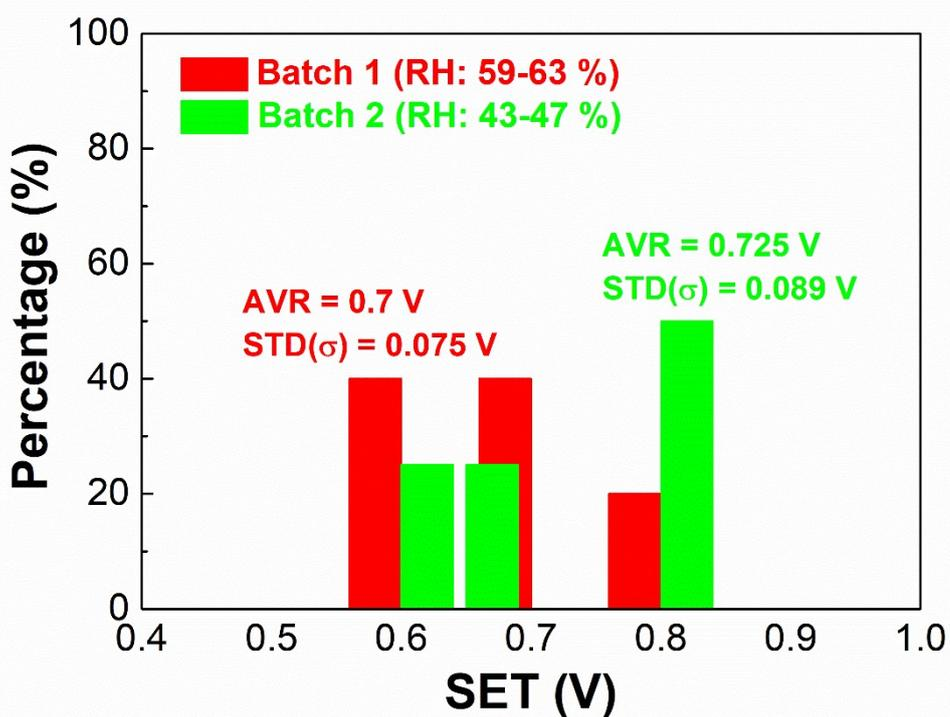
**Figure S10.** Histogram for the set voltage distribution for two batches under different relative humidity (RH) of the optimal memristors conditions.
