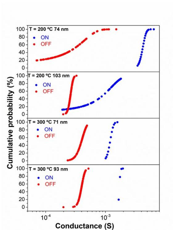
**Figure S9.** Conductance fluctuation of on and off states in each studied condition.
