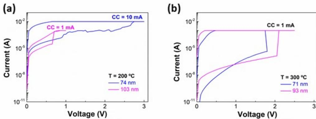
**Figure S7.** Electroforming I-V curves of the devices annealed at (a) 200 °C and (b) 300 °C.
