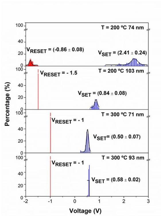
**Figure S8.** Set and reset average voltage of the I-V curves studied in each condition.
