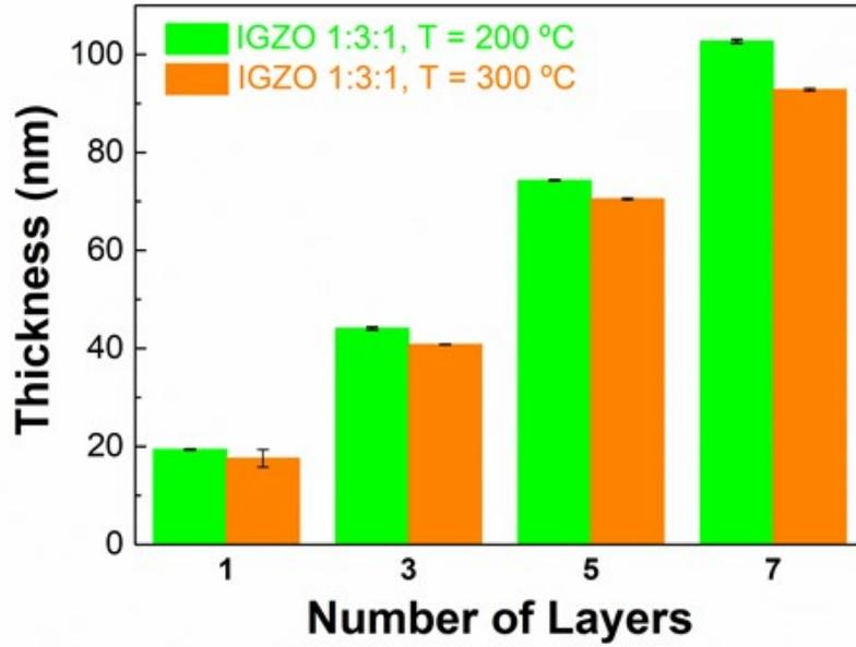
**Figure S6.** Spectroscopy measurements of the IGZO 1:3:1 thin films thickness (nm): annealed at 200 °C (light green), IGZO 1:3:1 at 300 °C (orange).
