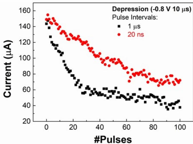
**Figure S12.** Conductance response, under a 0.1 V read voltage of 100 consecutive pulses with -0.8 V and 10  $\mu\text{s}$  with different pulse intervals.
