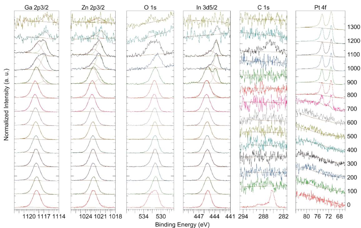
**Figure S4.** XPS cluster depth profile spectra of Ga 2p<sub>3/2</sub>, Zn 2p<sub>3/2</sub>, O 1s, In 5d<sub>3/2</sub>, C 1s and Pt 4f of a device annealed at 200 °C. The etch time in seconds is displayed on the right.
