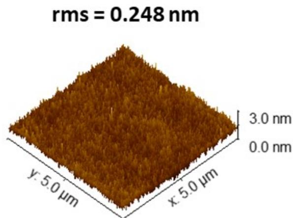
**Figure S3.** Three-dimensional AFM image ( $5 \times 5 \mu\text{m}^2$ ) of an IGZO thin film with  $\sim 90$  nm thickness and annealed at 300 °C deposited in a glass/Ti/Pt substrate.
