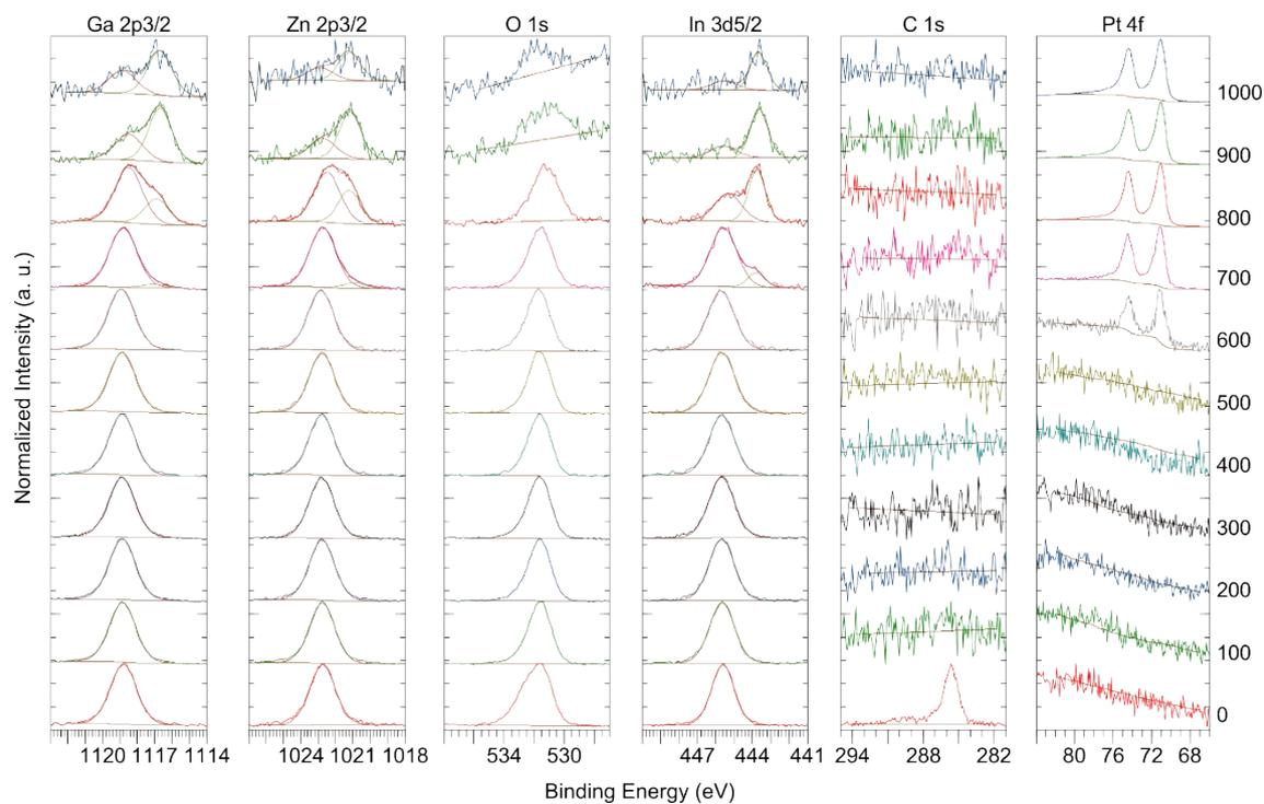
**Figure S5.** XPS cluster depth profile spectra of Ga 2p<sub>3/2</sub>, Zn 2p<sub>3/2</sub>, O 1s, In 5d<sub>3/2</sub>, C 1s and Pt 4f of a device annealed at 300 °C. The etch time is displayed on the right.
