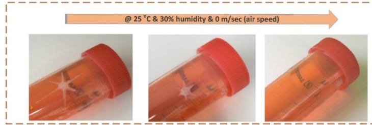
Figure S9. Degradability of the printed S-TENG using SSP technique. The degradation process of a star-shaped pattern, which shows the slow disappearance of the pattern over time and under ambient conditions of room temperature and 30% humidity.
