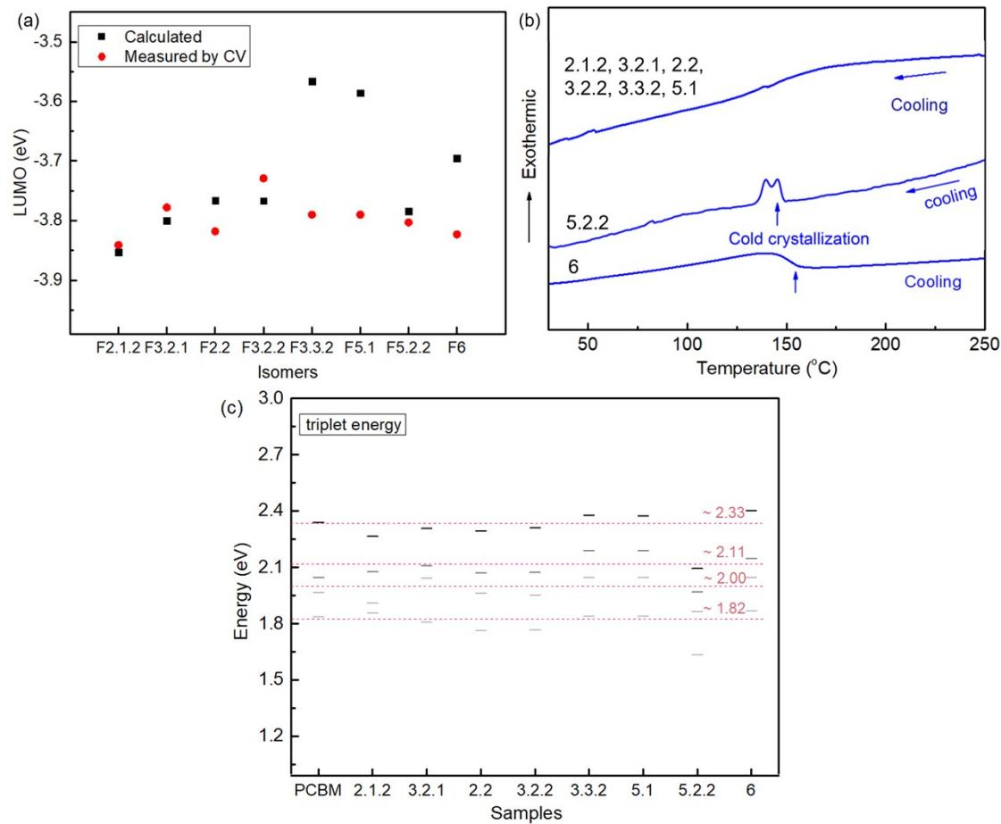
Fig. S1 (a) The isomer LUMO level statistics from Gaussian calculation and CV measurement. (b) Cooling process of the DSC test for different isomers. Isomers 2.1.2, 3.2.1, 2.2, 3.2.2, 3.3.2 and 5.1 show no crystallization peak and should be amorphous. Isomer 5.2.2 and 6 are relatively crystalline. (c) The calculated triplet energies (triplet state 1 to triplet state 4) of the isomers.
