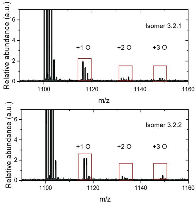
Fig. S3 MALDI-TOF measurement of bis-PCBM isomers 3.2.1 and 3.2.2 degraded in films under one sun in air for 60 mins.
