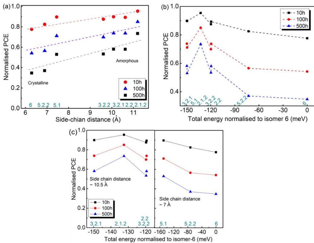
Fig. S9 Comparison between PCE and the fullerene molecular parameters of the burn-in degraded PCDTBT:bis-PCBM devices: (a) crystallinity and side-chain distance; (b) c) total energy.
