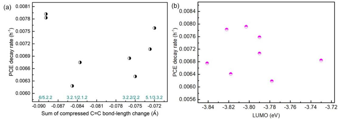
Fig. S10 Comparison between PCE decay rate and the fullerene molecular parameters of the burn-in degraded PCDTBT:bis-PCBM devices: (a) strain; (b) LUMO energy.
