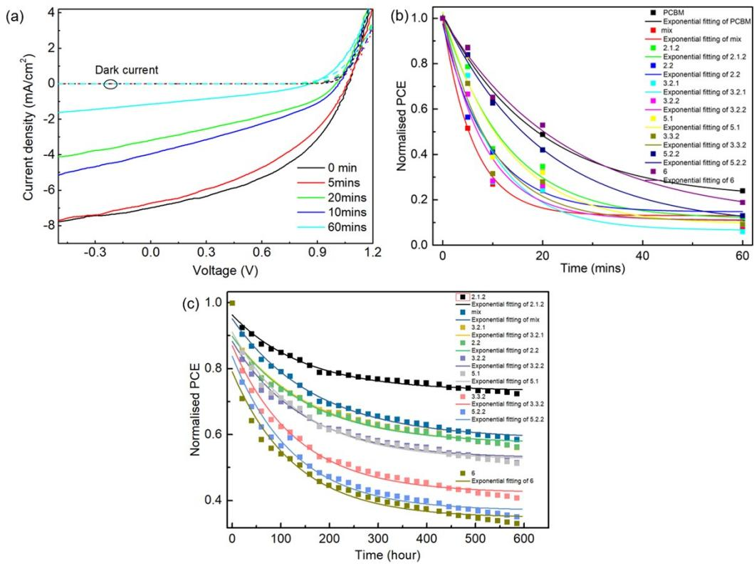
Fig. S4 (a) The typical  $J$ - $V$  curves of isomer 5.1 before and after photodegradation in air for different time. (b) The exponential fitting of degradation performance under light and air. (c) The exponential fitting of degradation performance under light and  $\text{N}_2$ .
