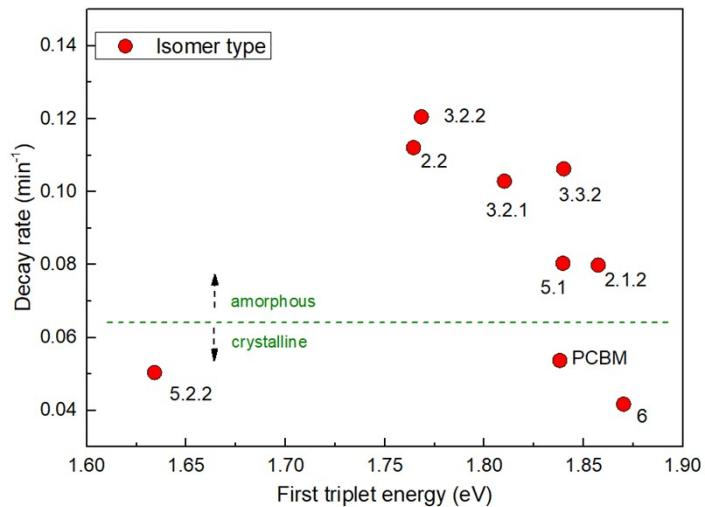
Fig. S6 Photodegradation rate of blend devices made with different fullerene isomers, plotted against calculated energy of the first triplet state. No correlation is evident within either the group of three crystalline fullerenes nor the group of 6 amorphous isomers.
