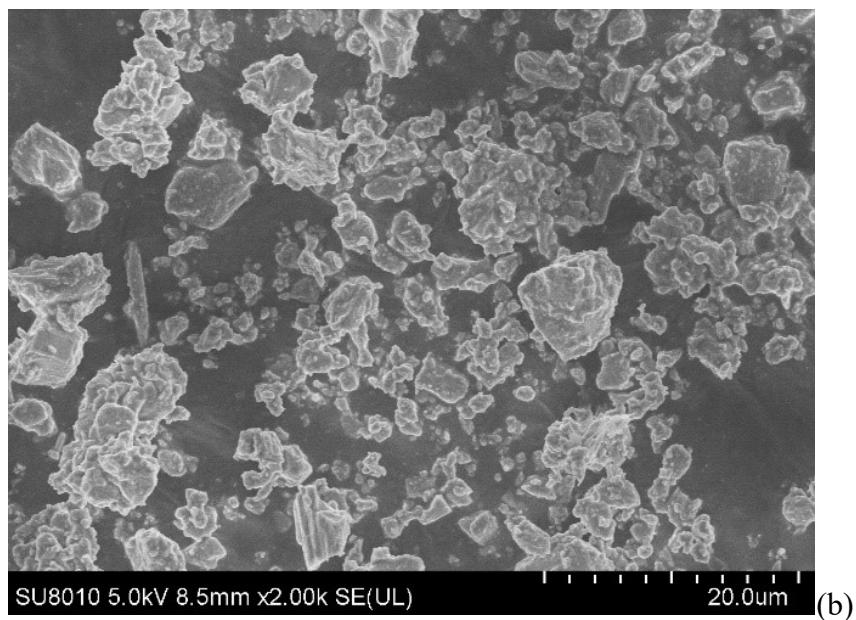
**Fig. S11** The SEM photo images of bulk and microscale crystals of [BPPP]SbCl<sub>5</sub>.
