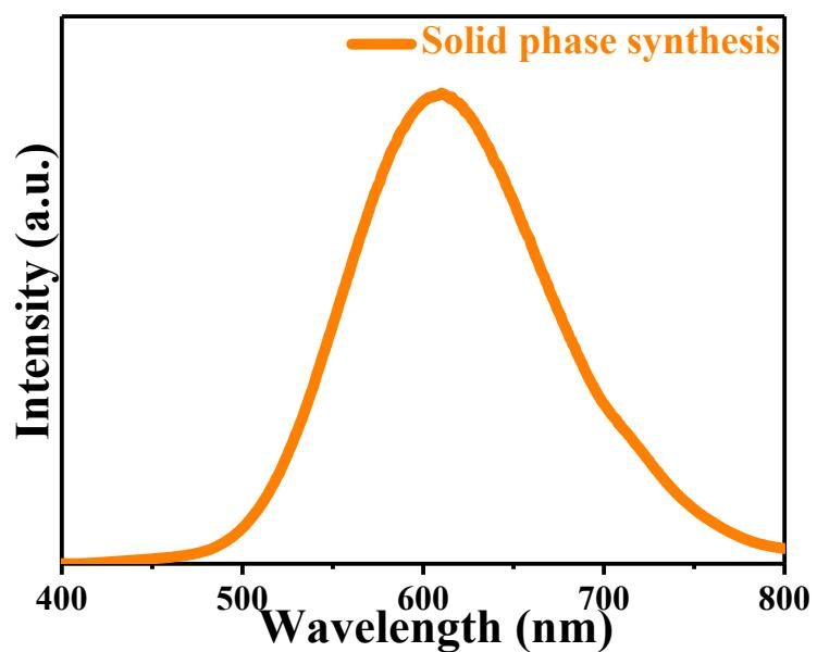
**Fig. S24** The PL emission spectrum of [BPPP]SbCl<sub>5</sub> prepared form mechanical grinding solid-state reaction.
