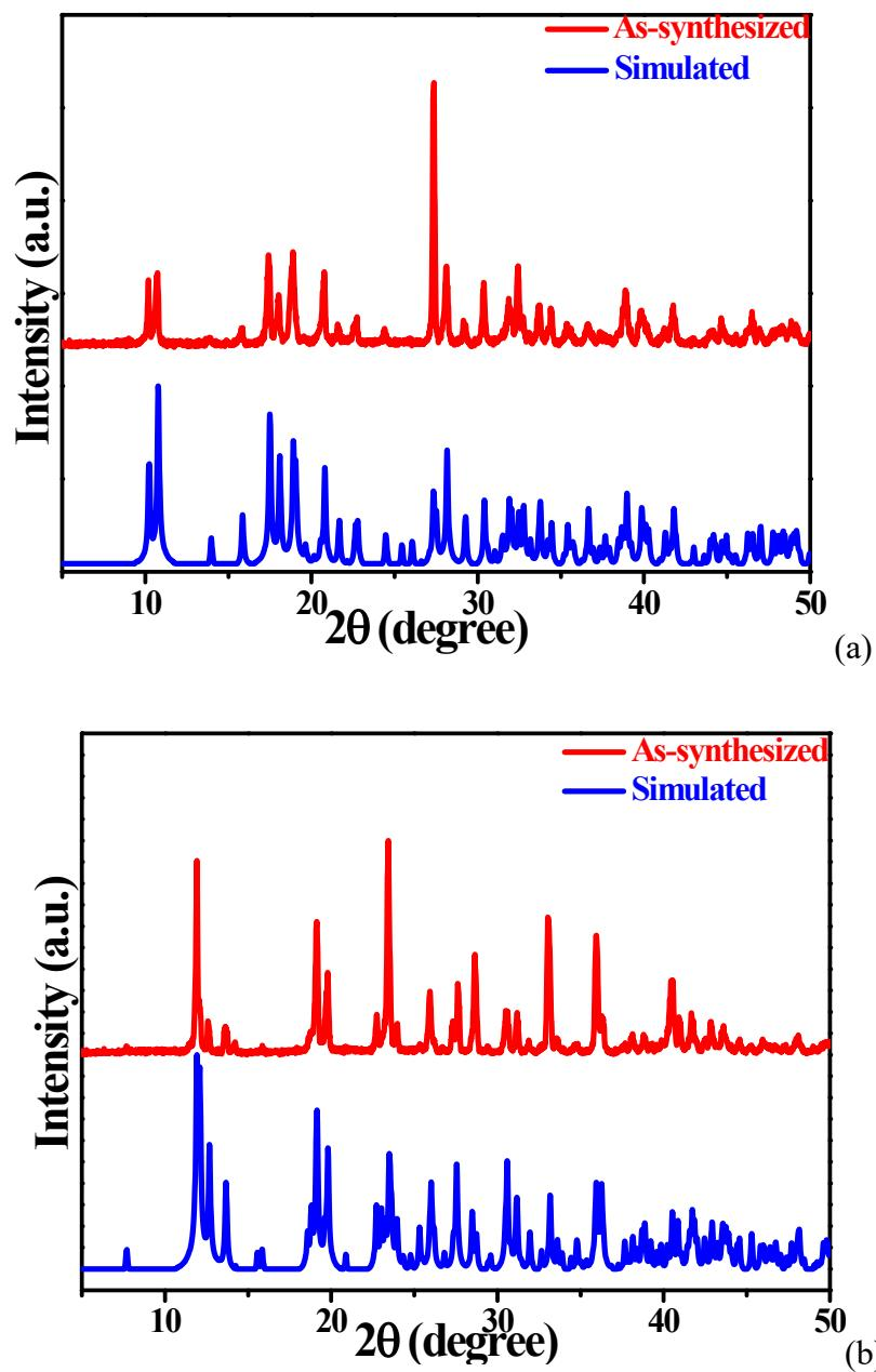
**Fig. S3** The experimental and simulated PXRD patterns of  $[BPP]SbCl_5$  (a) and  $[BPPP]SbCl_5$  (b).
