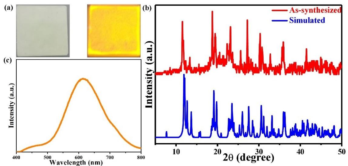
**Fig. S20** Normal characterizations of [BPPP]SbCl<sub>5</sub> based film: (a) photographs under ambient light and 365 nm UV light, (b) experimental PXRD pattern and simulated data and (c) PL emission spectrum.
