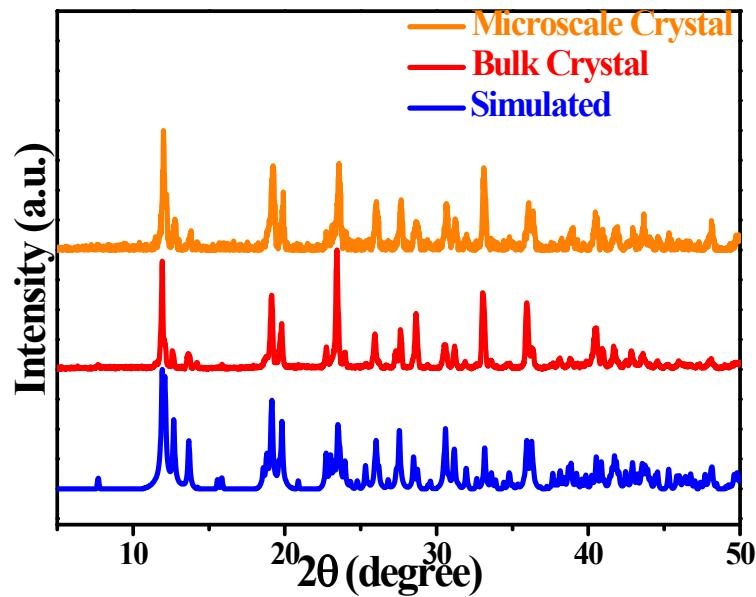
**Fig. S10** Experimetal PXRD patterns of bulk and microscale crystals as well as simulated data for [BPPP]SbCl<sub>5</sub>.
