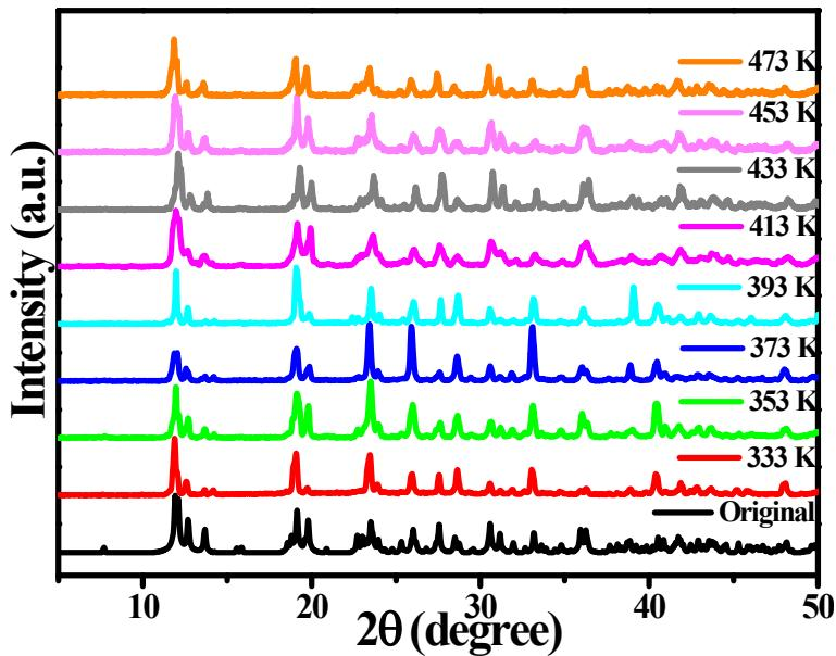
**Fig. S14** The experimental PXRD patterns of  $[BPPP]SbCl_5$  after constant heating at different temperature.
