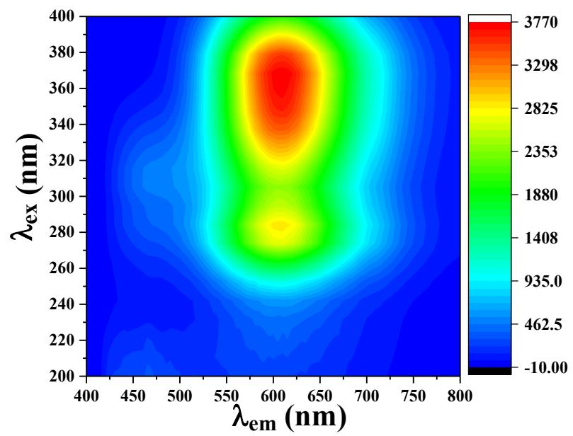
**Fig. S7** The 3D consecutive PL excitation and emission correlation map of  $[\text{BPPP}]\text{SbCl}_5$ .
