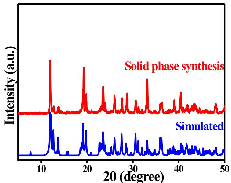
**Fig. S23** The experimental PXRD patterns of  $[BPPP]SbCl_5$  prepared from mechanical grinding solid-state reaction and simulated data from single crystal.
