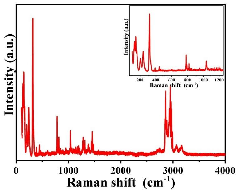
**Fig. S12** The Raman spectrum of [BPPP]SbCl<sub>5</sub>.
