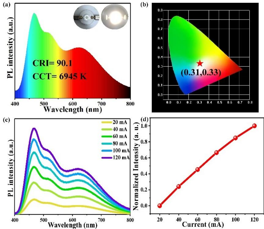
**Fig. S19** Characterizations of white LED fabricated by yellow [BPPP]SbCl<sub>5</sub> phosphor and blue phosphor BaMgAl<sub>10</sub>O<sub>17</sub>:Eu<sup>2+</sup> on a UV chip: a) The PL emission spectrum at 20 mA drive current (inset: photographs of fabricated white LED before and after switching power supply); b) the CIE chromaticity coordinates; c) drive current dependent PL emission spectra; d) the normalized peak intensity variation under various operating currents.
