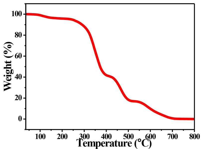
**Fig. S13** The thermogravimetric analysis of [BPPP]SbCl<sub>5</sub>.
