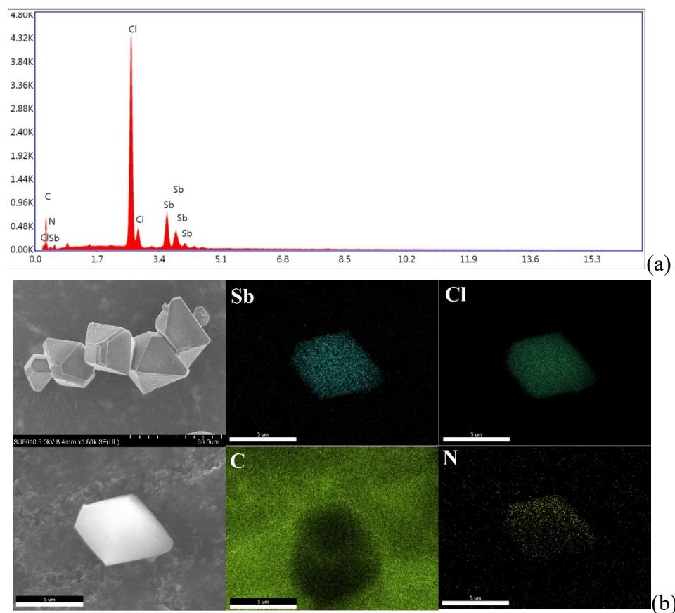
**Fig. S4** The energy dispersive X-Ray spectroscopy (EDX) analysis result (a) and SEM and elemental mapping images (b) of [BPPP]SbCl<sub>5</sub> bulk crystal.
