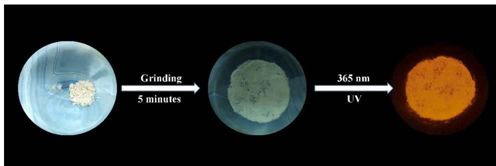
**Fig. S22** The photo images of mechanical grinding process of  $[BPPP]SbCl_5$  under the UV light irradiation.
