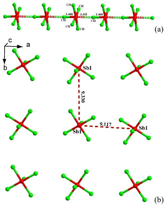
**Fig. S1** The detailed arrangement structures of  $[\text{SbCl}_5]^{2-}$  units in  $[\text{BPP}]\text{SbCl}_5$  (a) and  $[\text{BPPP}]\text{SbCl}_5$  (b).
