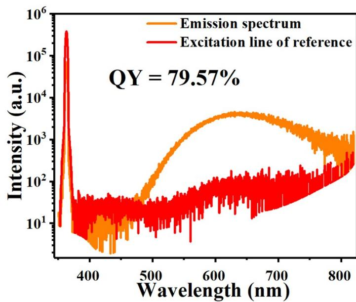
**Fig. S5** The PLQY of bulk crystals for compound [BPPP]SbCl<sub>5</sub>.
