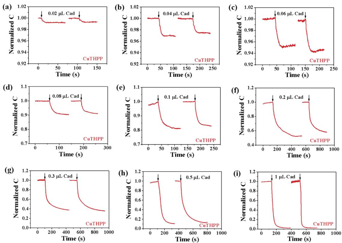
**Fig. S6** Normalized capacitance curves of IC-CuTHPP sensors to Cad of (a) 0.02, (b) 0.04, (c) 0.06, (d) 0.08, (e) 0.1, (f) 0.2, (g) 0.3, (h) 0.5, and (i) 1  $\mu\text{L}$ .
