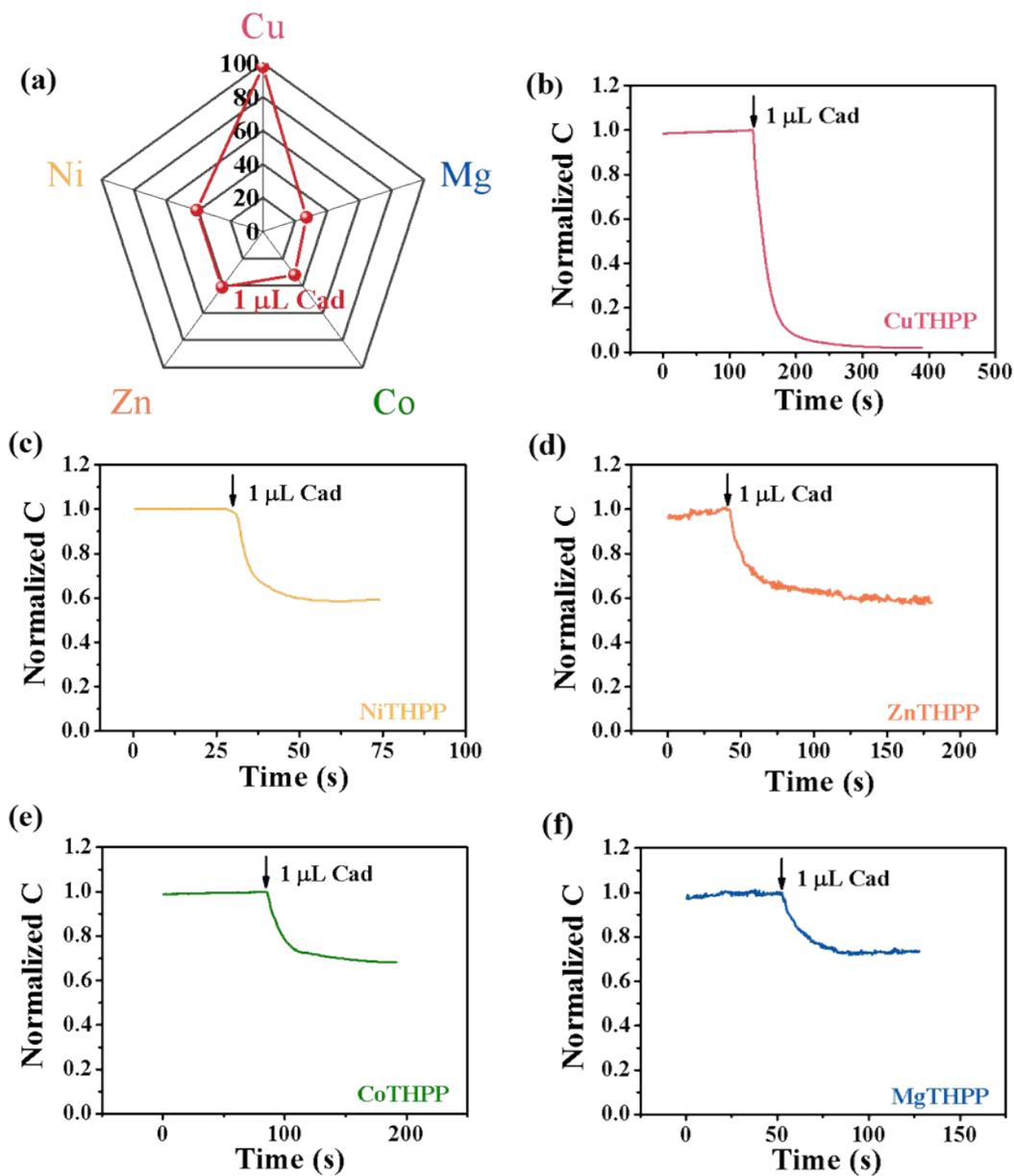
**Fig. S5** (a) Capacitance response of IC-MOFs sensors based on different metal ions to Cad of 1  $\mu\text{L}$ . (b) Normalized capacitance curve of IC-MOFs sensors based on CuTHPP, (c) NiTHPP, (d) ZnTHPP, (e) CoTHPP, and (f) MgTHPP to Cad of 1  $\mu\text{L}$ .
