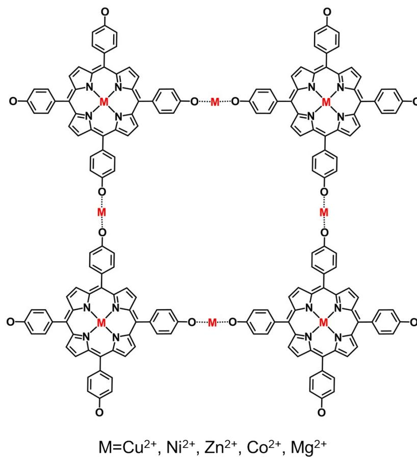
**Fig. S1** Chemical structures of IC-MOFs.
