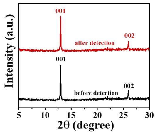
**Fig. S2** Out-of-plane XRD patterns of CuTHPP IC-MOF thin films before and after detection of Cad.
