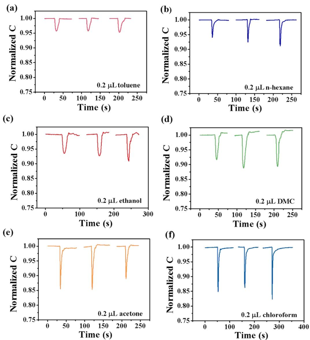
**Fig. S7** Normalized capacitance curves of IC-CuTHPP sensors to (a) toluene, (b) n-hexane, (c) ethanol, (d) DMC, (e) acetone, and (f) chloroform of 0.2  $\mu\text{L}$ .
