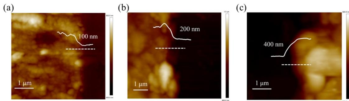
**Fig. S3** The AFM images of CuTHPP IC-MOF thin films. (a-c) MOF thin films of different thickness (100, 200, and 400 nm).
