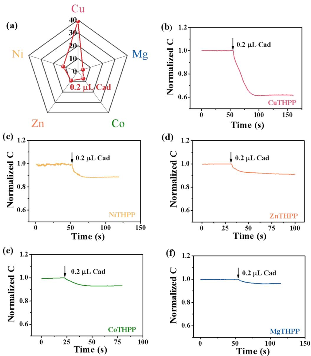
**Fig. S4** (a) Capacitance response of IC-MOFs sensors based on different metal ions to Cad of 0.2  $\mu\text{L}$ . (b) Normalized capacitance curve of IC-MOFs sensors based on CuTHPP, (c) NiTHPP, (d) ZnTHPP, (e) CoTHPP, and (f) MgTHPP to Cad of 0.2  $\mu\text{L}$ .
