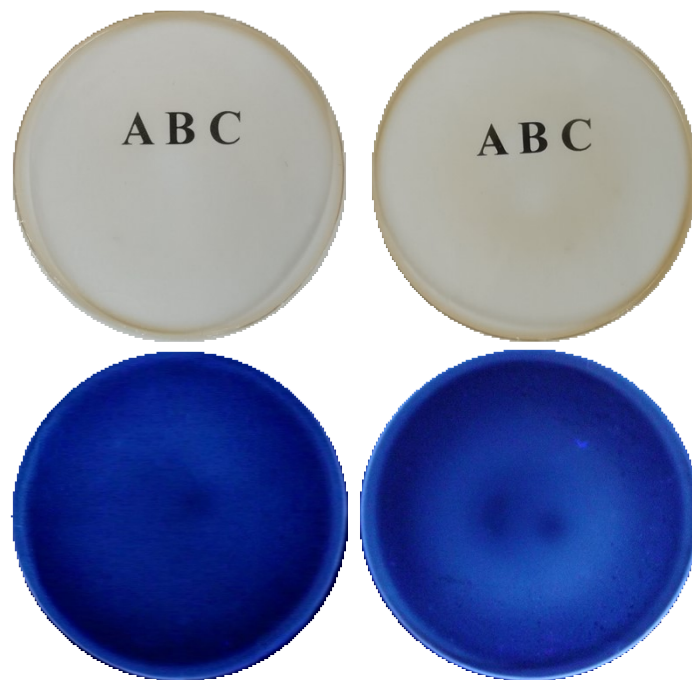
Fig. S7 Photos of the PMMA-based composite films containing 3.5 wt% (left) and 5.0 wt% (right) \alpha -Al-CDs, taken under room light (top) and 365 nm UV irradiation (bottom), respectively. Macroscopic phase separation is visible by naked eyes.
