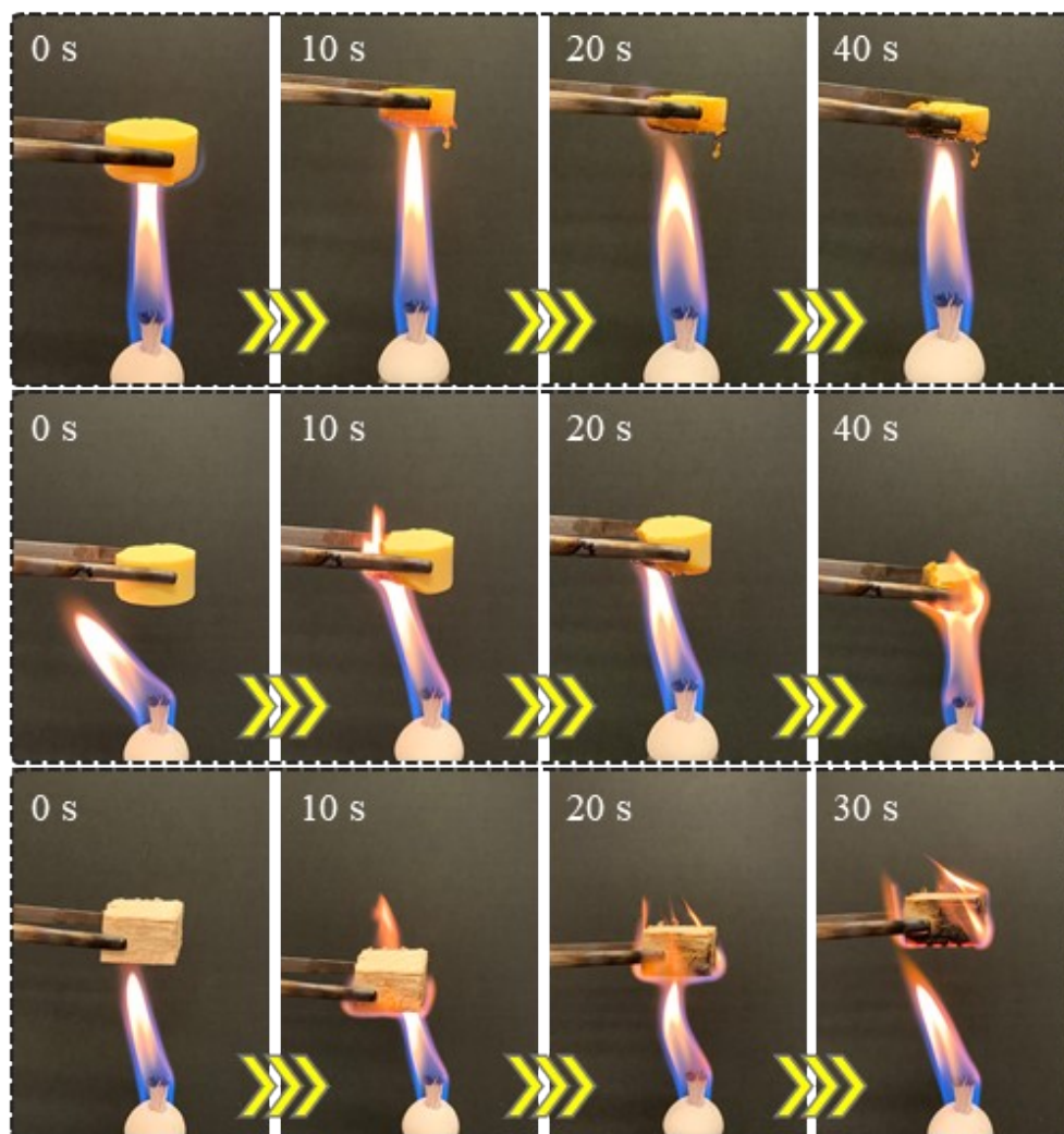
Figure S5. Flammability test of aerogels (S1M on the top and S2M in the middle) compared with the one for natural wood (on the bottom)
