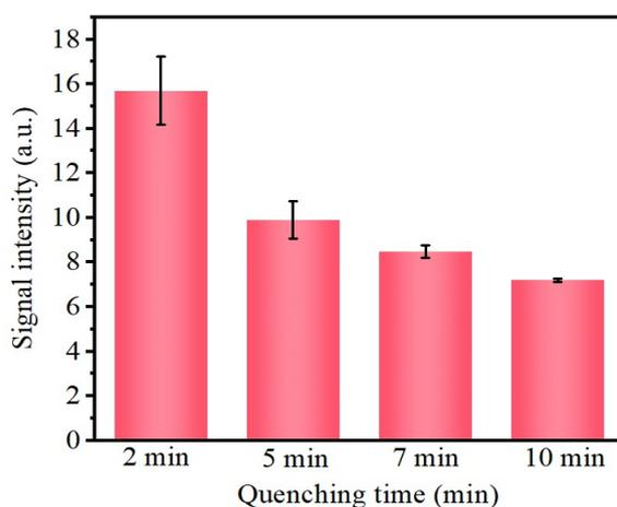
Fig. S2. The effect of quenching time on signal intensity; test conditions: 160 nM GR-5S-Cy3, 200 nM GR-5E-BHQ2 The error bars corresponded to the standard deviation of the data points in three repeated experiments (n = 3).
