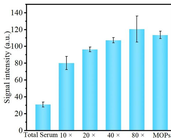
Fig. S5 Matrix effect of serum on the  $Pb^{2+}$  detection using the OFEWB; Testing condition:  $30^{\circ}C$ ,  $pH=7$ ,  $0.15 \text{ mol/kg}$  ionic strength,  $120 \text{ nM } Pb^{2+}$ ,  $160 \text{ nM GR-5S}$ ,  $200 \text{ nM GR-5E}$ . The error bars corresponded to the standard deviation of the data points in three repeated experiments ( $n = 3$ ).
