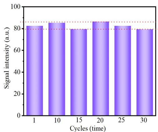
Fig. S6 The reusability of the OFEWB for the detection of  $Pb^{2+}$  in diluted serum. Testing condition:  $30^{\circ}C$ ,  $pH=7$ ,  $0.15 \text{ mol/kg}$  ionic strength,  $160 \text{ nM}$  GR-5S-Cy3,  $200 \text{ nM}$  GR-5E-BHQ2,  $80 \text{ nM}$   $Pb^{2+}$ . The error bars corresponded to the standard deviation of the data points in three repeated experiments ( $n = 3$ ).
