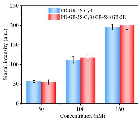
Fig. S4 The effects of the DNA length on  $Pb^{2+}$  detection using OFEWB. The error bars corresponded to the standard deviation of the data points in three repeated experiments ( $n = 3$ ).
