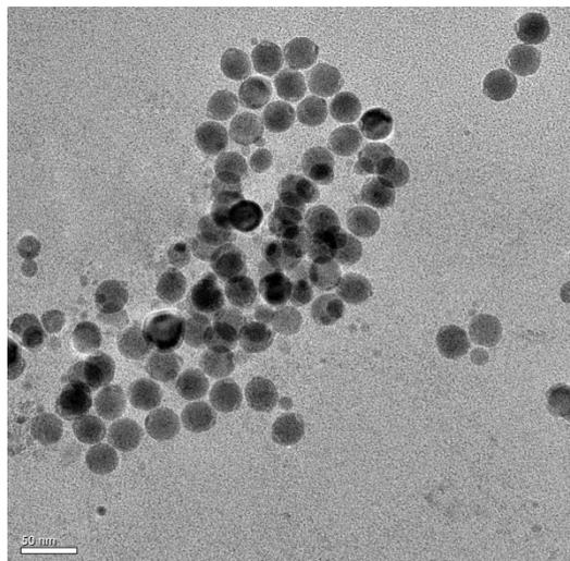
Figure S1 TEM image of  $\text{MnFe}_2\text{O}_4$  NPs.
