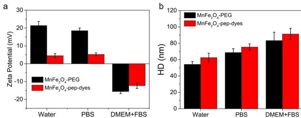
Figure S5 The zeta potentials and hydrodynamic diameters of as-prepared MnFe<sub>2</sub>O<sub>4</sub>-PEG and MnFe<sub>2</sub>O<sub>4</sub>-pep-dyes.
