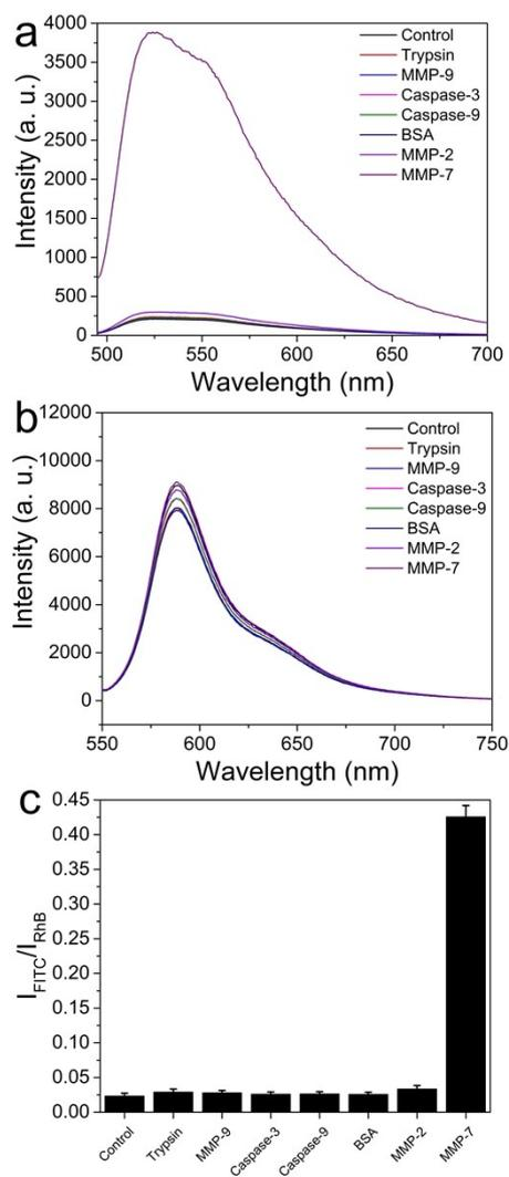
Figure S9 The selectivity of the nanoprobe. The fluorescence spectra of FITC (a) and RhB (b), and the relative  $I_{FITC}/I_{RhB}$  (c) after  $MnFe_2O_4$ -pep-dyes were incubated with different proteases and protein. The error bars mean standard deviations ( $n=3$ ).
