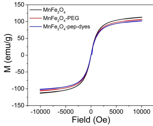
Figure S4 Magnetic Hysteresis loops of MnFe<sub>2</sub>O<sub>4</sub>-oleate, MnFe<sub>2</sub>O<sub>4</sub>-PEG, MnFe<sub>2</sub>O<sub>4</sub>-pep-dyes.
