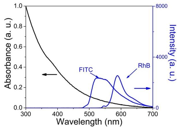
Figure S2 UV-visible spectrum of MnFe<sub>2</sub>O<sub>4</sub> NPs (black line) and fluorescence spectra of FITC-peptide and RhB-peptide (blue line).
