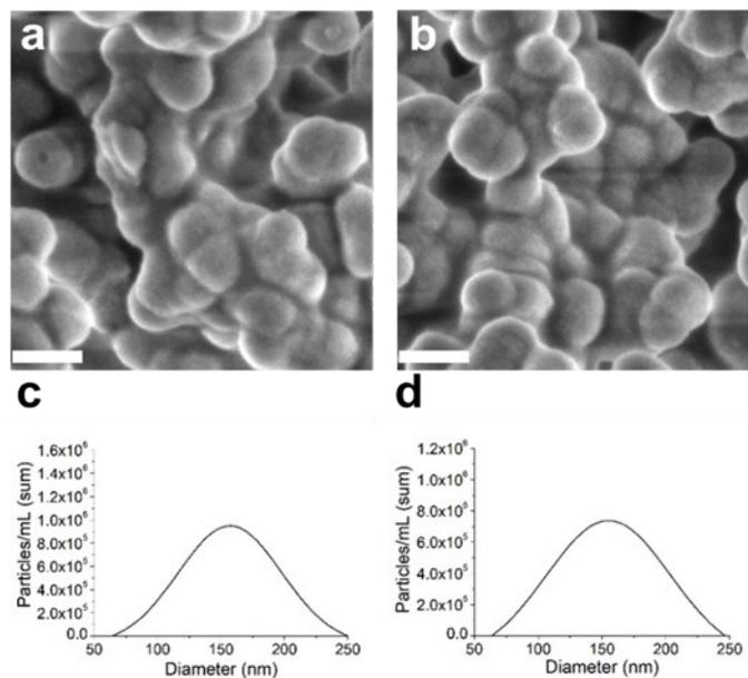
**Figure S3** FE-SEM images of (a) PPV@MSN-CP1@SLB, and (b) PPV@MSN-CP1@FA. Scale bar, 100 nm; NTA of (c) PPV@MSN-CP1@SLB, and (d) PPV@MSN-CP1@FA.
