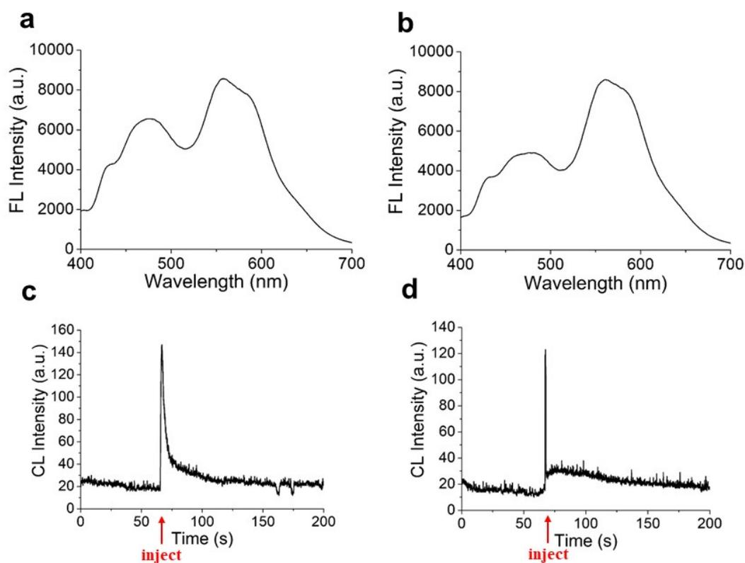
**Figure S7.** FL spectra of (a) 100  $\mu\text{g}/\text{mL}$  PPV@MSN-CP1@SLB ( $\lambda_{\text{ex}}=490$  nm) (b) 100  $\mu\text{g}/\text{mL}$  PPV@MSN-CP1@SLB@FA ( $\lambda_{\text{ex}}=490$  nm). CL of (c) 10  $\mu\text{g}/\text{mL}$  PPV@MSN-CP1@SLB (d) 10  $\mu\text{g}/\text{mL}$  PPV@MSN-CP1@SLB@FA. The FL spectra and the CL were measured in water. CL was induced by the addition of NaClO (50 mM).
