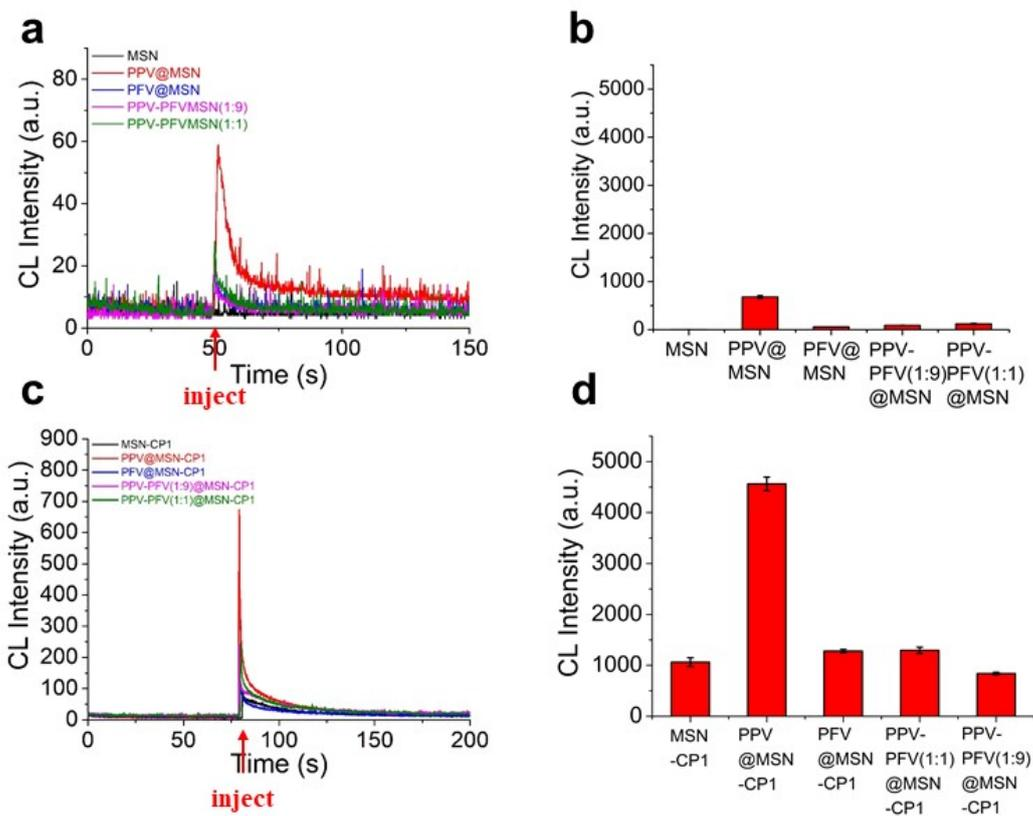
**Figure S6.** CL spectra of (a) 10  $\mu\text{g/mL}$  PPV/PFV@MSN, and (c) 10  $\mu\text{g/mL}$  PPV/PFV@MSN-CP1. Quantification of the CL of (b) 10  $\mu\text{g/mL}$  PPV/PFV@MSN and (d) 10  $\mu\text{g/mL}$  PPV/PFV@MSN-CP1. The CL was measured in ethanol. CL was induced by the addition of NaClO (50 mM). The error bars represent the standard deviations ( $n = 3$ ). The spectra were measured in ethanol.
