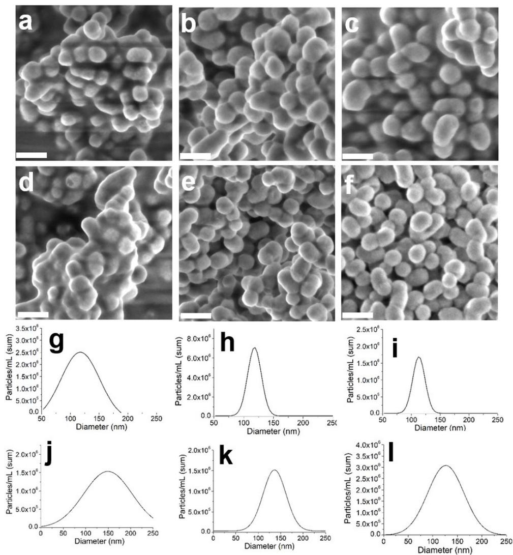
**Figure S2** FE-SEM images of (a) PFV@MSN, (b) PPV@PFV(1:1)@MSN, (c) PPV-PFV(1:9)@MSN, (d) PFV@MSN-CP1, (e) PPV-PFV(1:1)@MSN-CP1, and (f) PPV-PFV(1:9)@MSN-CP1. Scale bar, 100 nm; NTA of (g) PFV@MSN, (h) PPV-PFV(1:1)@MSN, (i) PPV-PFV(1:9)@MSN, (j) PFV@MSN-CP1, (k) PPV-PFV(1:1)@MSN-CP1, and (l) PPV-PFV(1:9)@MSN-CP1.
