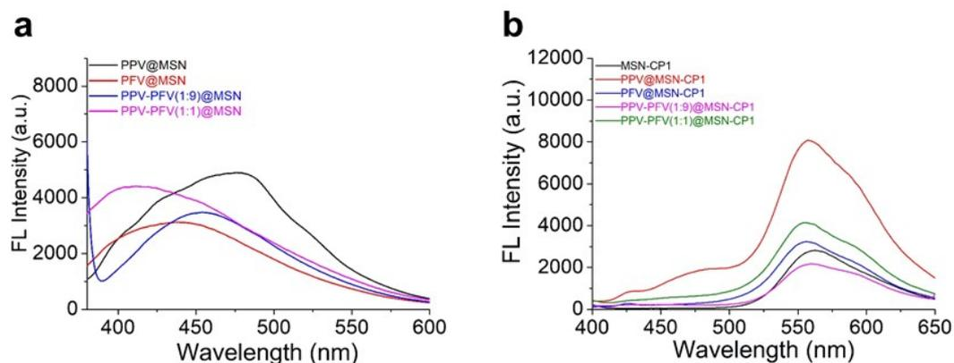
**Figure S5.** Fluorescence spectra of (a) 100  $\mu\text{g/mL}$  PFV@MSN ( $\lambda_{\text{em}}=430$  nm), PFV-PPV(1:1)@MSN ( $\lambda_{\text{em}}=420$  nm), PFV-PPV(9:1)@MSN ( $\lambda_{\text{em}}=460$  nm), and (b) 100  $\mu\text{g/mL}$  PPV/PFV@MSN-CP1 ( $\lambda_{\text{em}}=560$  nm). The spectra were measured in ethanol.
