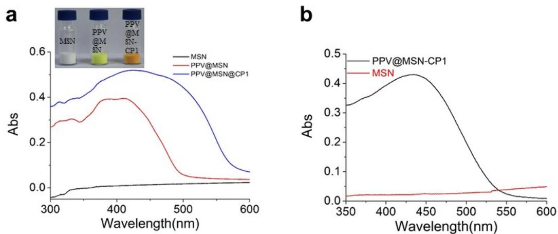
**Figure. S4** UV-Vis absorption spectra of (a) MSN(black) PPV@MSN(red) PPV@MSN-CP1(blue) and (b) PPV@MSN-CP1(after etching)
