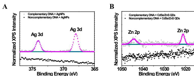
Fig S2, A) Zn 2p region XPS spectra of the PAP interface after hybridization with AgNPs labelled with target DNA and non-target DNA; B) Zn 2p region XPS spectra of the PAP interface after hybridization with CdSe/ZnS QDs labelled with target DNA and non-target DNA.
