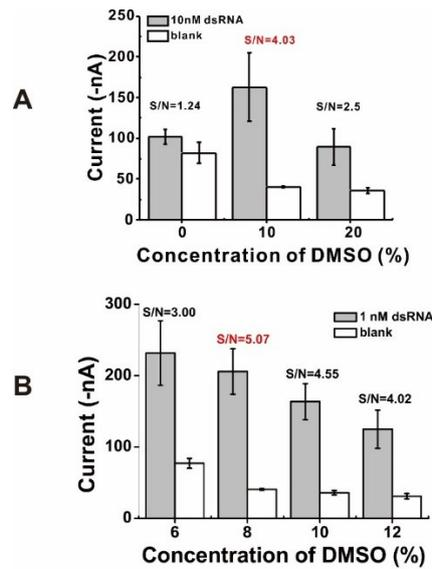
Figure S3. The analysis results of E-biosensors with different concentrations of DMSO in the pre-hybridization solution. The target RNA concentration was: A) 1 nM, B) 1 nM.
