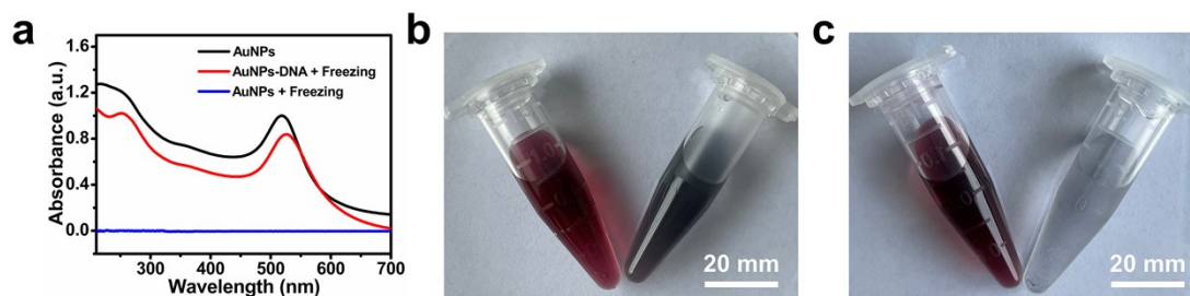
Figure S9. (a) The UV-vis absorption spectra of AuNPs + Freezing, AuNPs, and AuNPs-DNA + Freezing. (b) The images of AuNPs-DNA (left) and AuNPs (right) after addition of 1 M NaCl. (c) The images of AuNPs-DNA + Freezing (left) and AuNPs + Freezing (right) after addition of 1 M NaCl.
