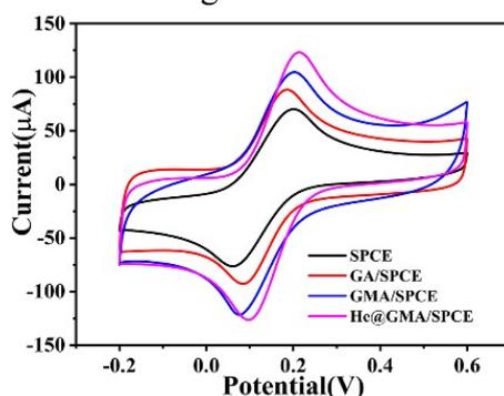
Fig. S2 CV curves recorded in 5 mM  $[\text{Fe}(\text{CN})_6]^{3-/4-}$ .
