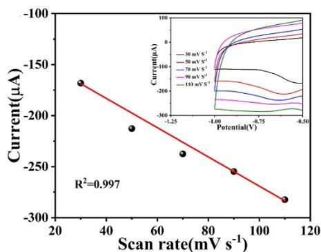
Fig. S3 Plot of reduction current versus scan rate in PBS containing 2 mM  $\text{H}_2\text{O}_2$ . Inset is the enlarged CV curves obtained at different scan rates.
