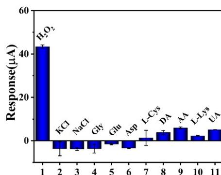
Fig. S4 Current responses of the chip towards 200  $\mu\text{M}$   $\text{H}_2\text{O}_2$  and 1 mM interferents (n=3).
