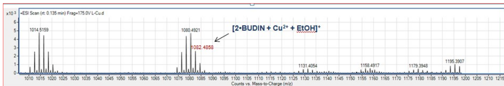
Fig S18. TOF MS spectrum of the complex of BUDIN – \text{Cu}^{2+}
