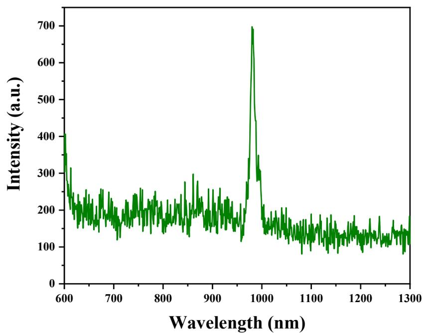
**Figure. S11** The fluorescence excitation spectra of oleic acid capped UCNPs ( $\text{NaYF}_4$ , Yb/Er) dispersed in cyclohexane.
