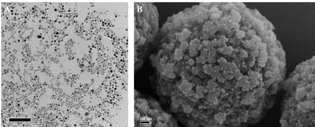
**Figure. S10** TEM images of (A) cDNA-UCNPs after stored in refrigerator at 4°C for one week; (B) MBs-DNA-cDNA-UCNPs after stored in refrigerator at 4°C for one week.
