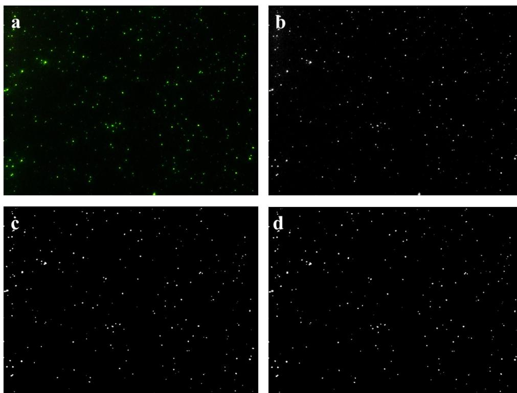
**Figure S1.** Images processing. (a) captured fluorescence images; (b) Image conversion to 8-bit format; (c) images after setting the pixel threshold; (d) images after setting the threshold for connected field area and used for counting.
