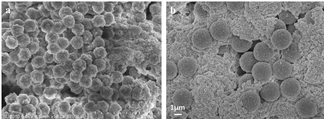
**Figure.S9** SEM images of (a) Improper control of the relationship between the amount ratio of DNA-MBs and cDNA-UCNPs for constructing biosensors; (b) Improper control of buffer salt concentration for constructing biosensors.
