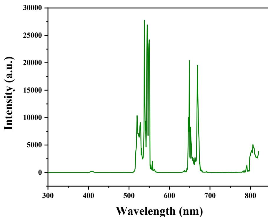
**Figure. S14** The fluorescence emission spectra of oleic acid shedding UCNP (NaYF<sub>4</sub>, Yb/Er) dispersed in ultrapure water.
