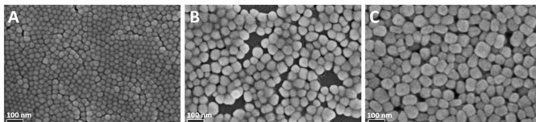
**Figure S3.** Different sizes of UCNPs under different time and temperature regulated. (A) ~30nm, heating for 1 hour under 305°C; (B) ~65nm, heating for 1.5 hours under 305°C; (C) ~105nm, heating for 1.5 hours under 310°C.
