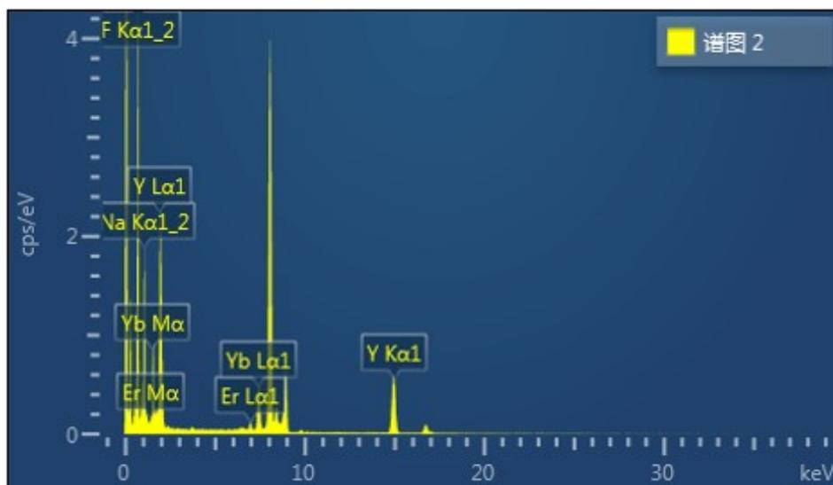
**Figure S4.** EDS Spectrogram of synthesized UCNPs.
