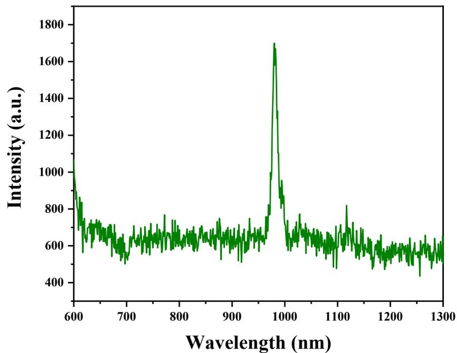
**Figure. S12** The fluorescence excitation spectra of oleic acid shedding UCNPs ( $\text{NaYF}_4$ , Yb/Er) dispersed in ultrapure water.
