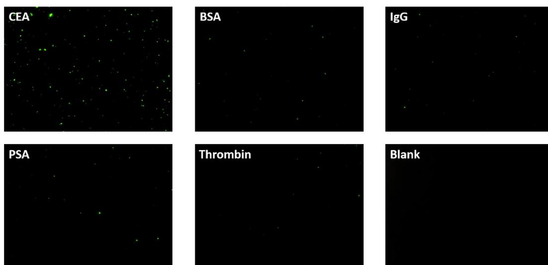
**Figure S15.** Representative upconversion microscopy images of cDNA-UCNPs on the coverslip surface in the presence of different proteins.
