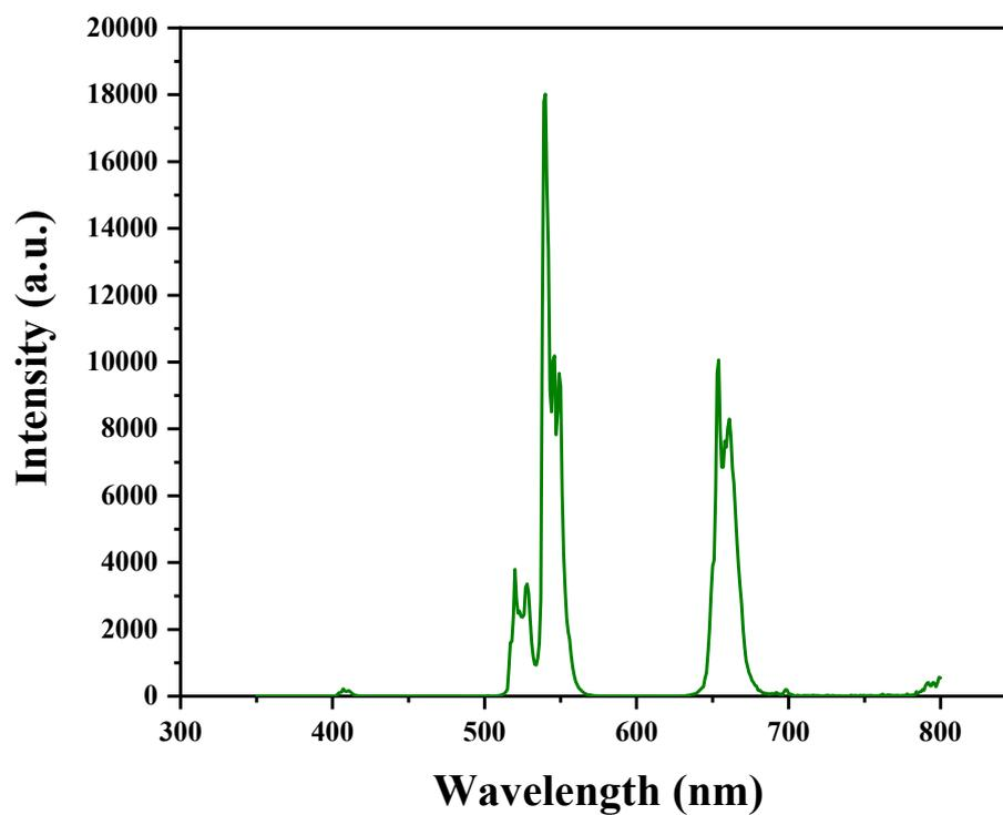
**Figure. S13** The fluorescence emission spectra of oleic acid capped UCNPs ( $\text{NaYF}_4$ , Yb/Er) dispersed in cyclohexane.
