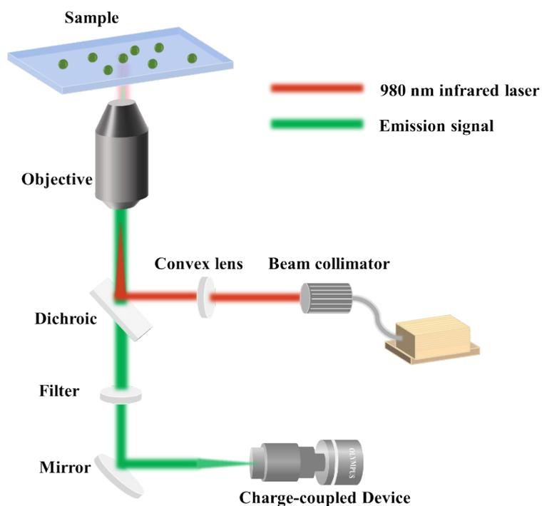
**Figure S2.** The construction diagram of the inverted fluorescence microscope we modified.
