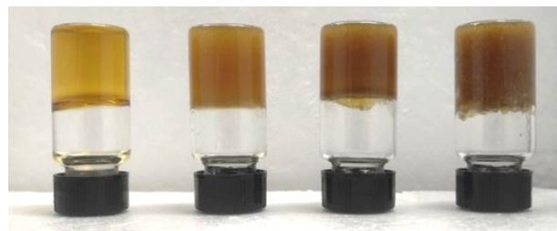
**Fig. S3.** The impact of different  $\text{Al}^{3+}$  (from left to right: 0, 0.02, 0.04, 0.10g) contents on gelation of the GA-containing samples.
