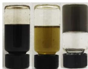
**Fig. S6.**  $\text{Al}^{3+}$  in P-0.3C-0.06GA-0.08Al was replaced by equal molar amount of  $\text{Fe}^{3+}$ ,  $\text{Cu}^{2+}$  and  $\text{Cr}^{3+}$  (from left to right), making P-0.3C-0.06GA-0.086Fe, P-0.3C-0.06GA-0.051Cu and P-0.3C-0.06GA-0.085Cr hydrogels. Only the gelation of P-0.3C-0.06GA-0.085Cr succeeded.
