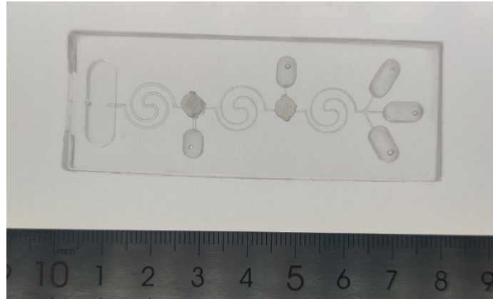
Fig. S2. The construction of Casade Fermat Spiral Microfluidic Chip. Assembly drawing of the fabricated push valve, cured dual PDMS layer.
