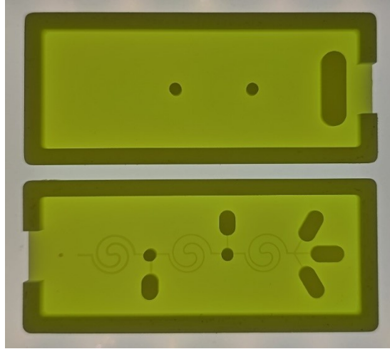
Fig. S1. The molds of dual PDMS layers are manufactured by SLA 3D printer.
