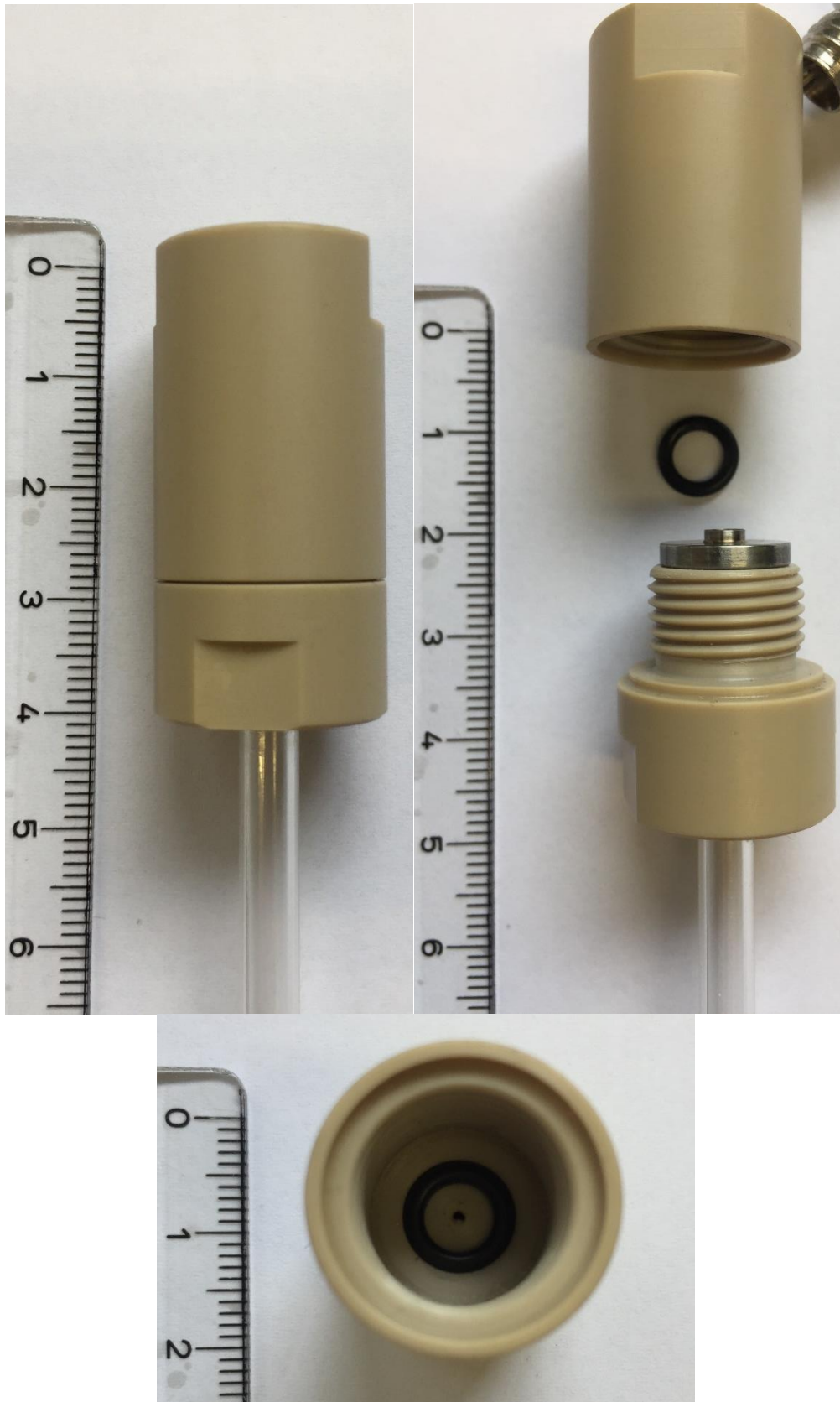
Figure SI3: Detailed photographs of the PEEK attachment for the sapphire tube. Top: PEEK attachment connected (left) and unscrewed (right). Bottom: inside of the top attachment with the rubber O-ring in place.
