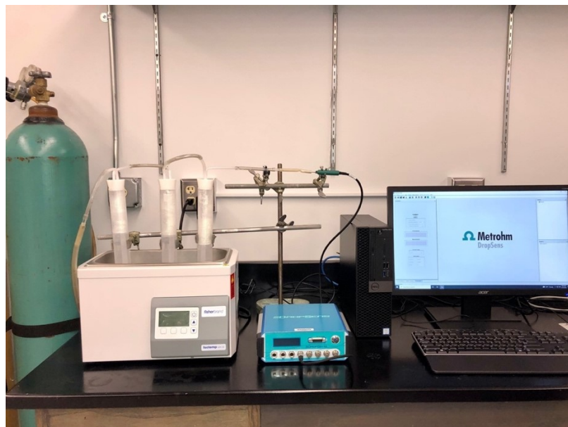
Figure S2. Setup for gas phase studies using SPEs, including potentiostat with SPE connection, computer with DropSens software, nitrogen gas tank, and water bath containing gas washing bottles.
