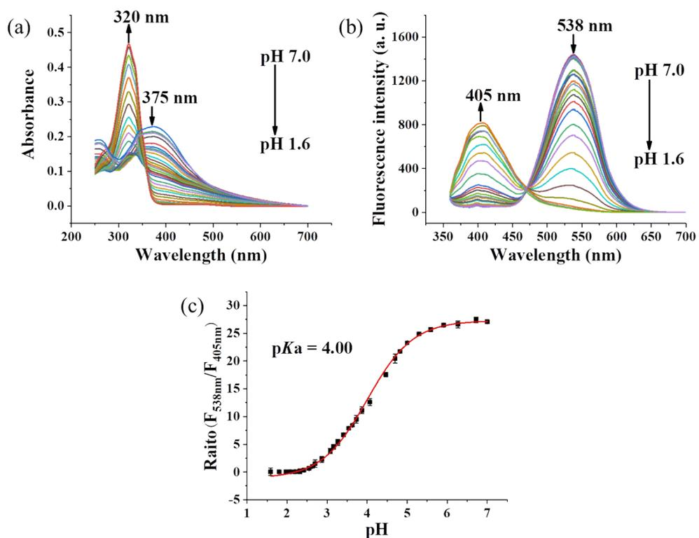
**Fig. S9** The optical performance of **OD**. (a) The absorption spectra of **OD** (10 μM) in a solution of pH 7.0-1.6. (b) The fluorescence spectra of **OD** (10 μM) in a solution of pH 7.0-1.6,  $\lambda_{\text{ex}} = 350$  nm. (c) The pH (7.0-1.6) dependent Raito ( $F_{538\text{nm}}/F_{405\text{nm}}$ ) sigmoidal fitting graph. Error bars represent standard deviation, n=5.
