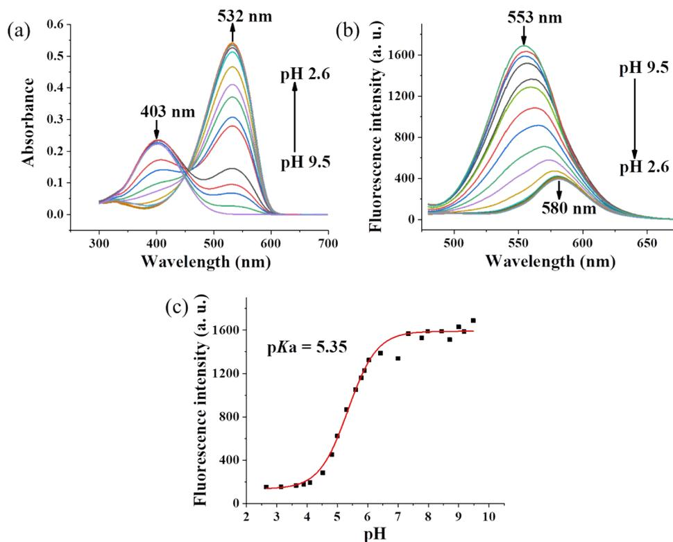
**Fig. S10** The optical performance of **ID**. (a) The absorption spectra of **ID** (10 μM) in a solution of pH 9.5-2.6. (b) The fluorescence spectra of **ID** (10 μM) in a solution of pH 9.5-2.6,  $\lambda_{\text{ex}} = 450$  nm. (c) The pH (9.5-2.6) dependent fluorescence intensity (553 nm) sigmoidal fitting graph. Error bars represent standard deviation, n=5.
