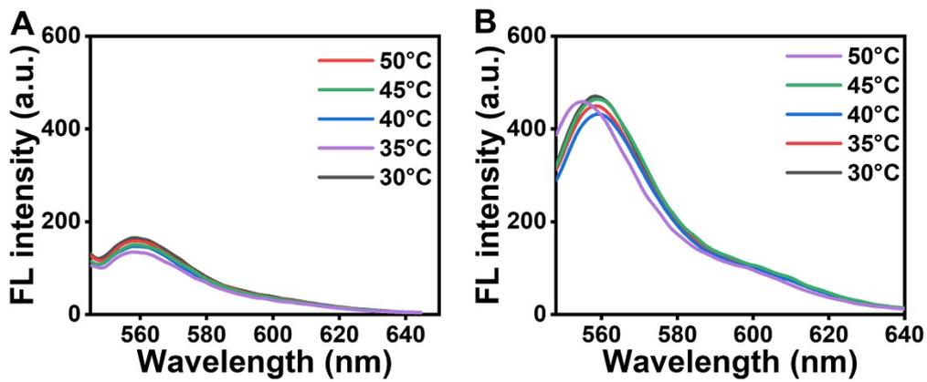
**Fig. S11** Fluorescence spectra of Au@SiO<sub>2</sub> NFs in the absence (A) or presence (B) of 1 mM miRNA-21 at different reaction temperatures.
