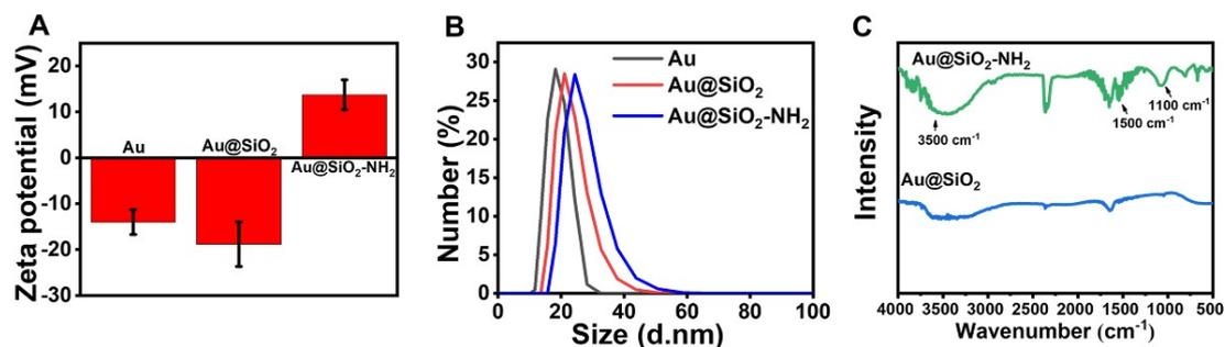
**Fig. S2** (A) Zeta-potentials of AuNPs, Au@SiO<sub>2</sub> and Au@SiO<sub>2</sub>-NH<sub>2</sub>. (B) Hydrodynamic size distribution of AuNPs, Au@SiO<sub>2</sub> and Au@SiO<sub>2</sub>-NH<sub>2</sub>. (C) FT-IR spectra of Au@SiO<sub>2</sub> and Au@SiO<sub>2</sub>-NH<sub>2</sub>.
