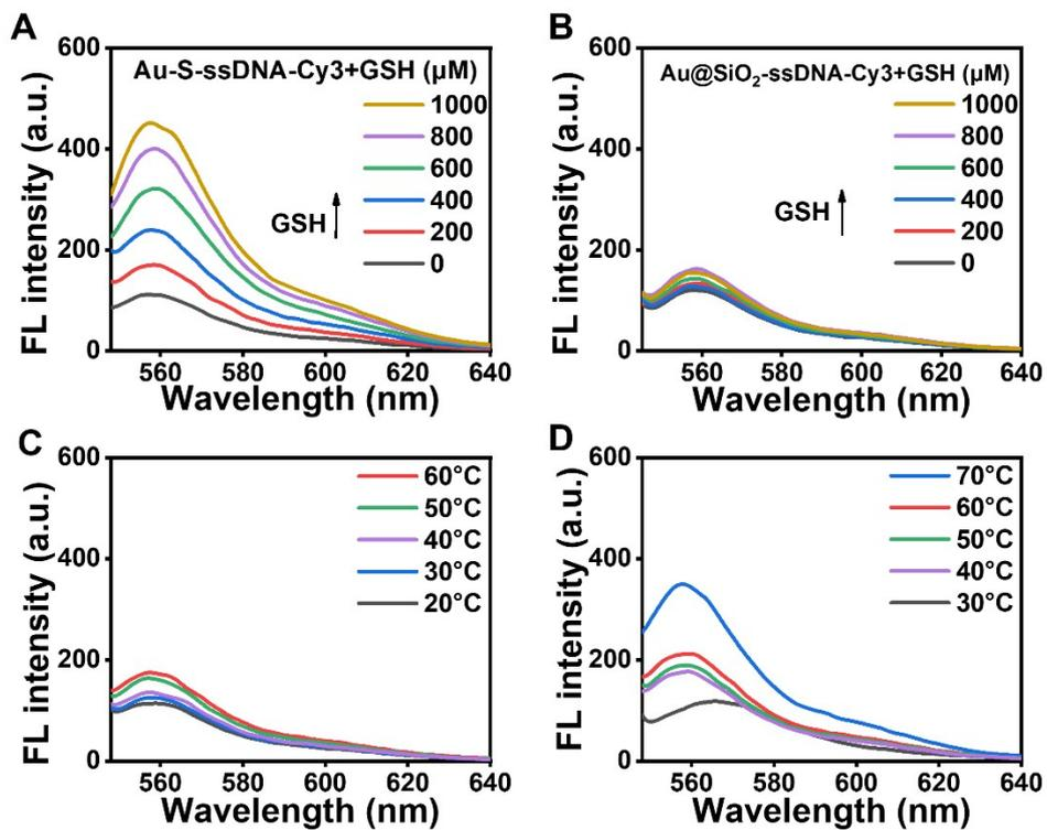
**Fig. S6** (A, B) Fluorescence spectra of Au-S-ssDNA-Cy3 (A) and Au@SiO<sub>2</sub>-ssDNA-Cy3 (B) in PBS buffer treating with different concentrations of GSH for 12 h. (C, D) Fluorescence spectra of Au@SiO<sub>2</sub>-ssDNA-Cy3 (C) and Au-S-ssDNA-Cy3 (D) after being treated at different temperatures for 12 h.
