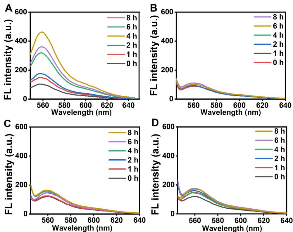
**Fig. S5** (A, B) Time-dependent fluorescence spectra of Au-S-ssDNA-Cy3 in the presence (A) and absence (B) of GSH (1 mM) at 37 °C. (C, D) Fluorescence spectra of Au@SiO<sub>2</sub>-ssDNA-Cy3 in PBS buffer with (C) and without (D) GSH (1 mM).
