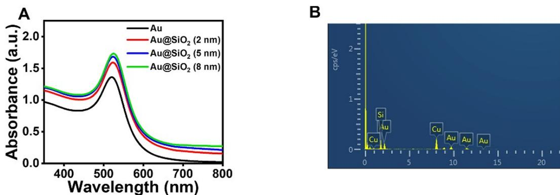
**Fig. S1** (A) UV-vis spectra of AuNPs and Au@SiO<sub>2</sub>. (B) EDS of Au@SiO<sub>2</sub>.
