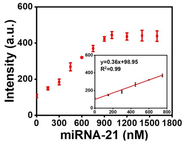
**Fig. S10** Fluorescence intensities of the Au-S NFs at different miRNA-21 concentrations. Inset: Linear calibration curve.
