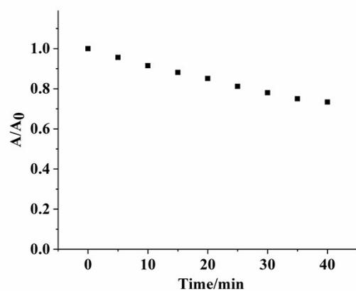
**Figure S6.** Time-dependent absorbance changes of probe **Naph-DFOB** (10.0  $\mu\text{M}$ ) under a Xe lamp irradiation (light intensity: 200  $\text{mW}/\text{cm}^2$ ) in PBS buffer (10.0 mM, pH = 7.4, containing 50% EtOH).
