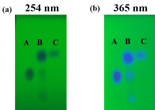
**Fig. S1.** TLC analysis of **NaphOH-CN** (A), the mixture of **NaphOH-CN** and  $\text{ClO}^-$  (B), and **NaphOH-CN-Cl** (C) under a UV lamp ((a):254 nm; (b): 365 nm). Stationary phase: silica gel. Solvent: petroleum ether: ethyl acetate = 3:1 (V/V).
