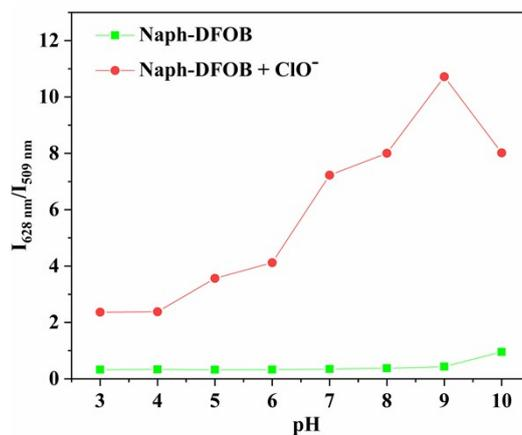
**Figure S5.** Fluorescence intensity ratio ( $I_{628 \text{ nm}}/I_{509 \text{ nm}}$ ) of **Naph-DFOB** (10.0  $\mu\text{M}$ ) in response to  $\text{ClO}^-$  (500.0  $\mu\text{M}$ ) at different pH value. Excitation wavelength: 430 nm. Test media: PBS buffer (10.0 mM, pH = 7.4, containing 50% EtOH).
