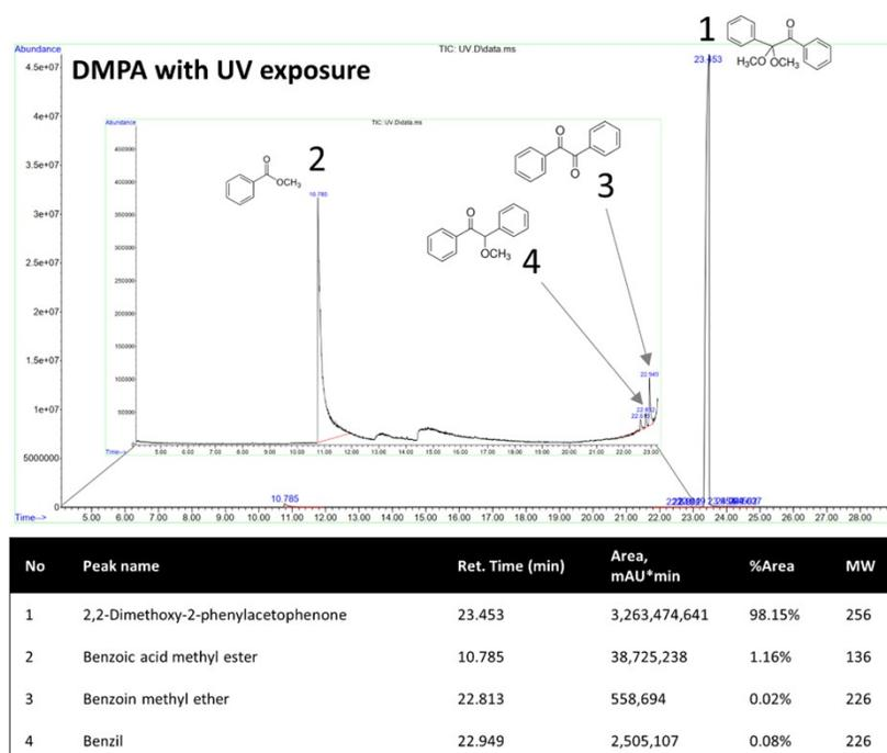
**Supplementary Fig. 1.** GC-MS data for identified products in DMPA with (top spectrogram) and without (bottom spectrogram) UV exposure. Identified peaks are summarized in the table below the respective spectrograms.
