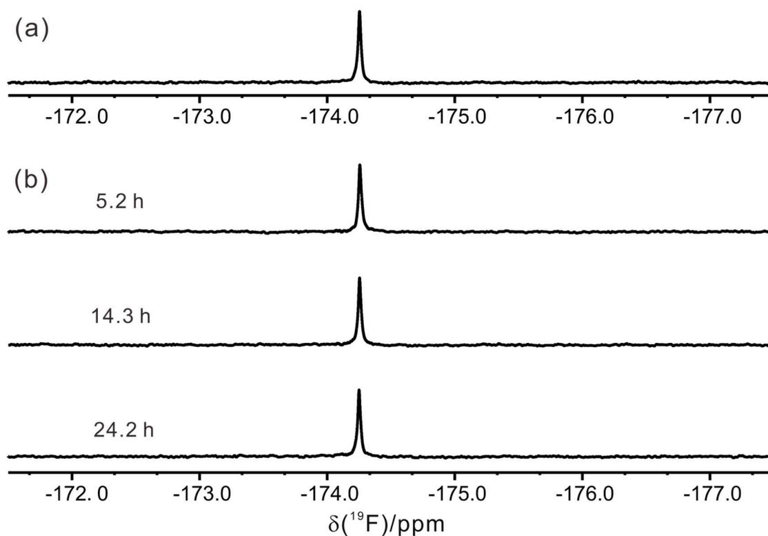
**Figure S6.** (a) The  $^{19}\text{F}$ -NMR spectra of the  $^{19}\text{F}$ -tag. (b) Time-dependent of  $^{19}\text{F}$ -NMR spectra recorded for the mixture of the  $^{19}\text{F}$ -tag and (*R*)-(+)-*N*-alpha-dimethylbenzylamine at 35 °C in  $\text{CDCl}_3$ . The concentrations of the  $^{19}\text{F}$ -tag and (*R*)-(+)-*N*-alpha-dimethylbenzylamine were 1.0 mM. The proton-decoupled  $^{19}\text{F}$ -NMR spectra were recorded at a magnetic field with a  $^{19}\text{F}$  frequency of 376 MHz.
