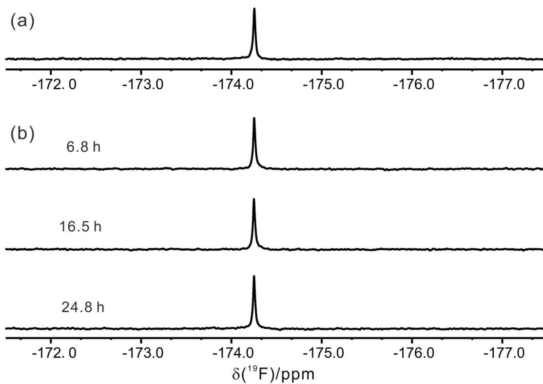
**Figure S7.** (a) The  $^{19}\text{F}$ -NMR spectra of the  $^{19}\text{F}$ -tag. (b) Time-dependent of  $^{19}\text{F}$ -NMR spectra recorded for the mixture of the  $^{19}\text{F}$ -tag and *N,N*-dimethylbenzylamine at 35 °C in  $\text{CDCl}_3$ . The concentrations of the  $^{19}\text{F}$ -tag and *N,N*-dimethylbenzylamine was 1.0 mM. The proton-decoupled  $^{19}\text{F}$ -NMR spectra were recorded at a magnetic field with a  $^{19}\text{F}$  frequency of 376 MHz.
