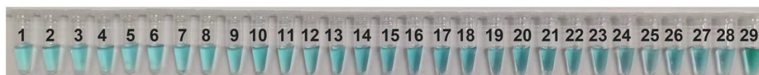
Fig. S12 The photographs of the specificity analysis of the glucose detection. The concentration of the interfering species, and glucose was 150 \mu\text{M} .
