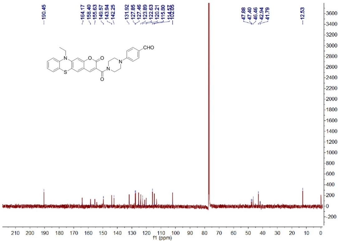
The  $^{13}\text{C}$  NMR (151 MHz) spectra of **Compound 7** in  $\text{CDCl}_3$ .
