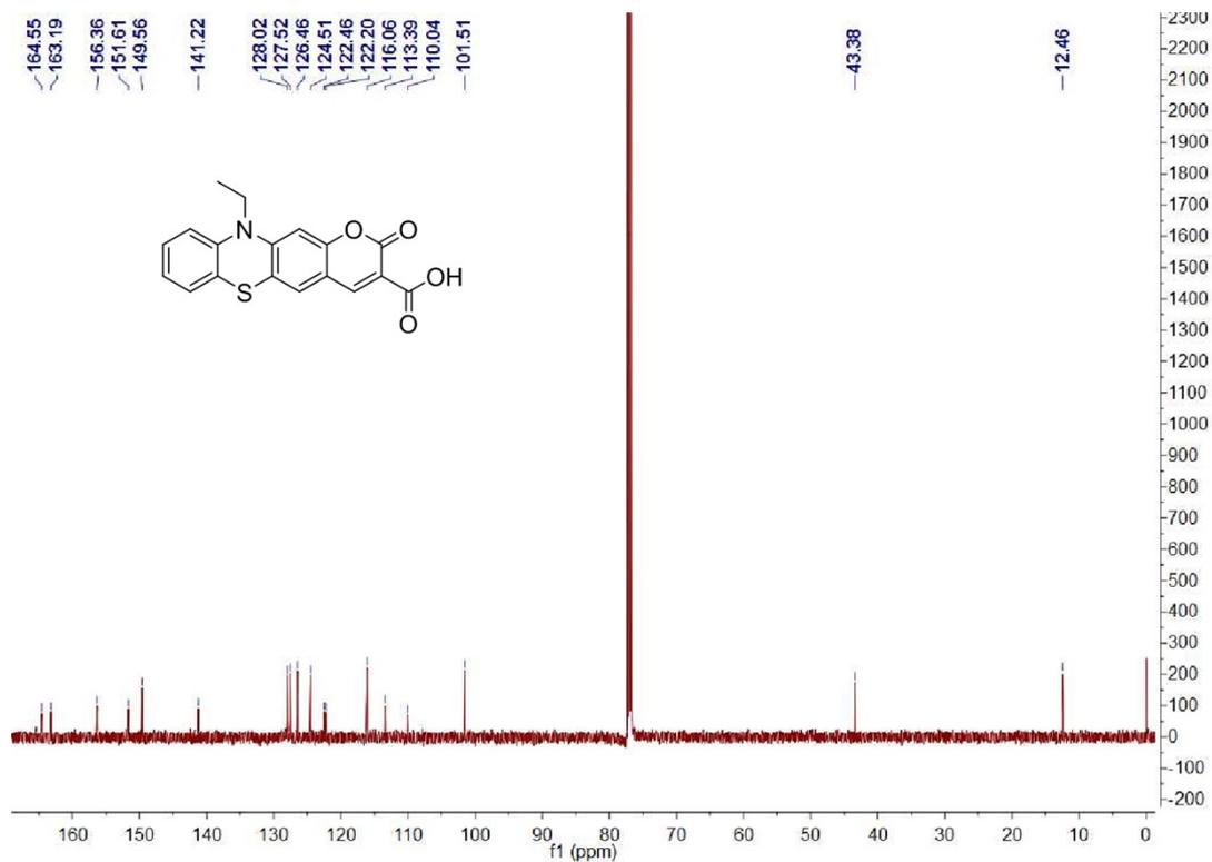
The  $^{13}\text{C}$  NMR (151 MHz) spectra of **Compound 5** in  $\text{CDCl}_3$ .
