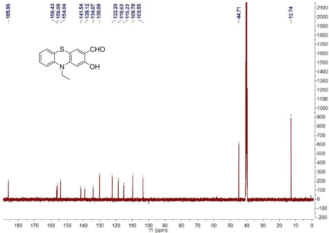
The  $^{13}\text{C}$  NMR (151 MHz) spectra of **Compound 3** in  $\text{DMSO-}d_6$ .
