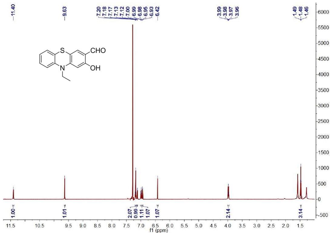
The  $^1\text{H}$  MNR (600 MHz) spectra of **Compound 3** in  $\text{CDCl}_3$ .
