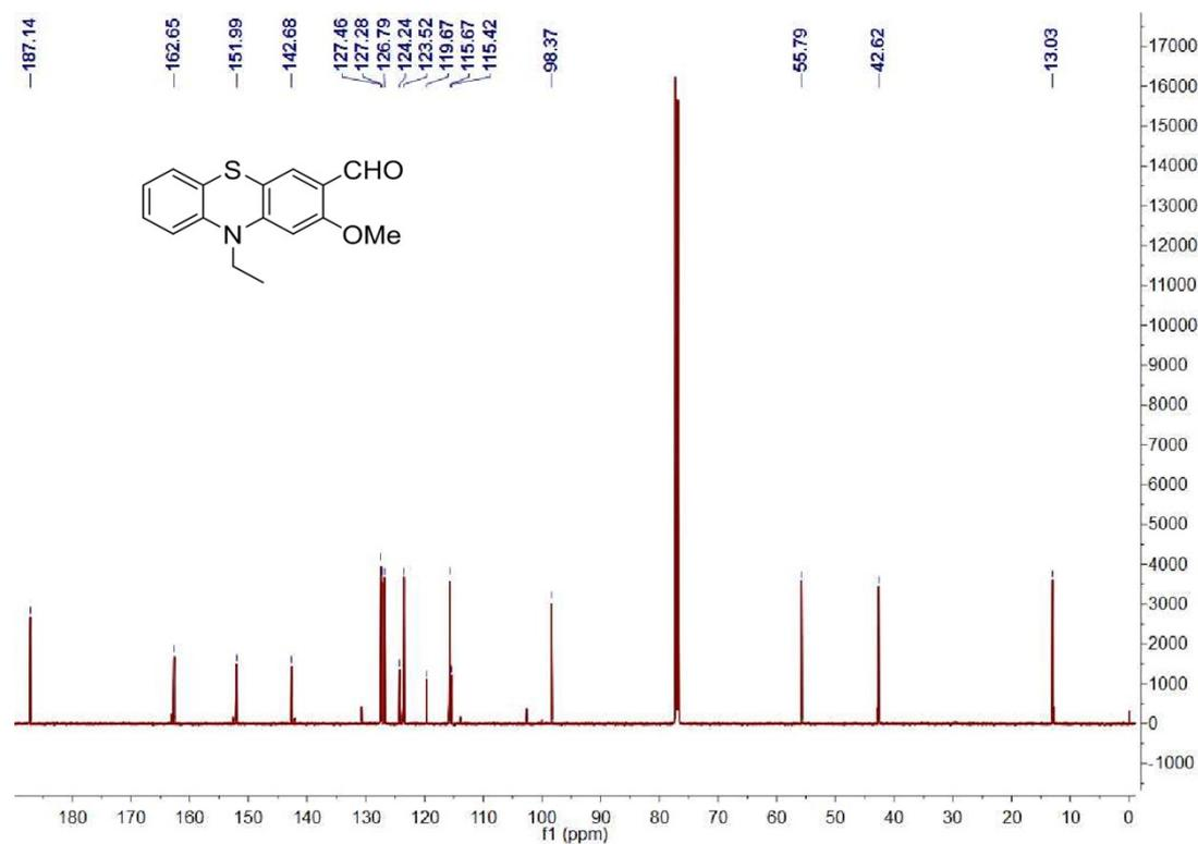
The  $^{13}\text{C}$  NMR (151 MHz) spectra of **Compound 2** in  $\text{CDCl}_3$ .
