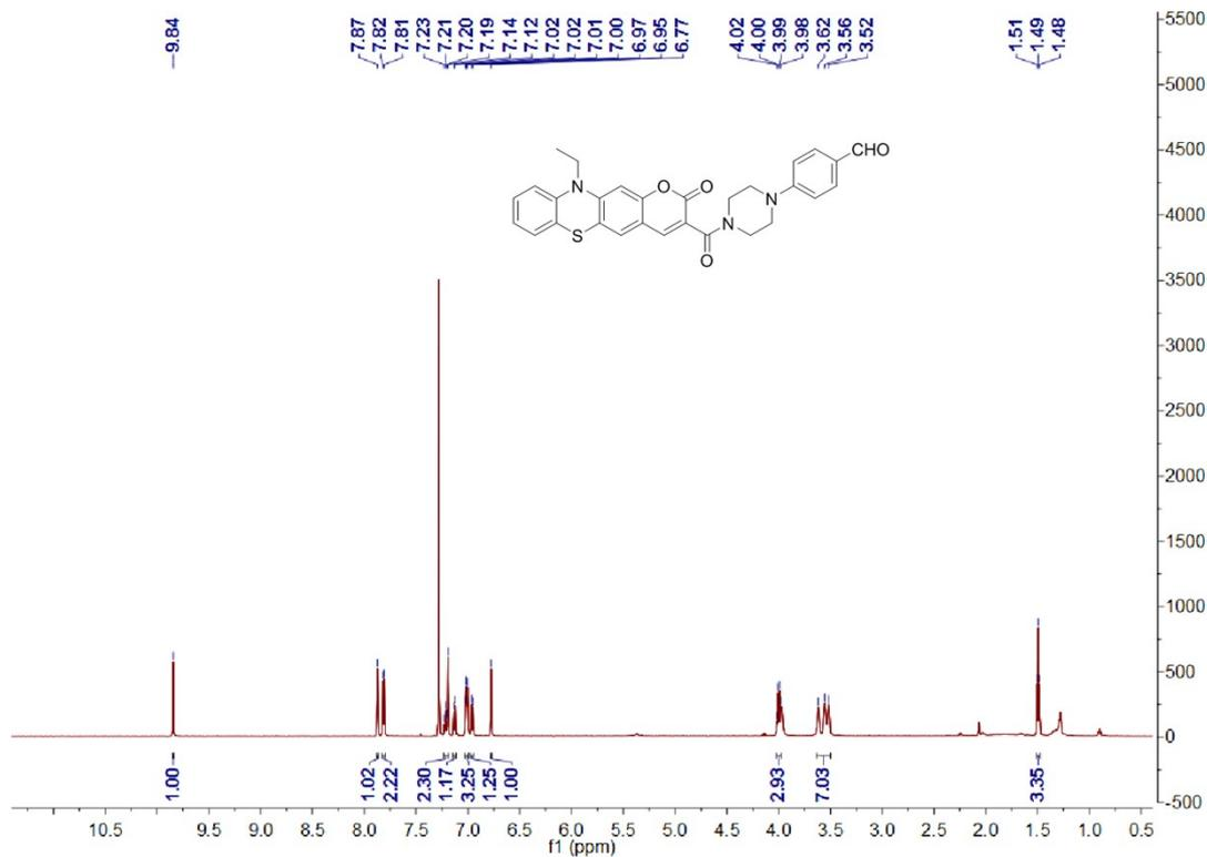
The  $^1\text{H}$  MNR (600 MHz) spectra of **Compound 7** in  $\text{CDCl}_3$ .
