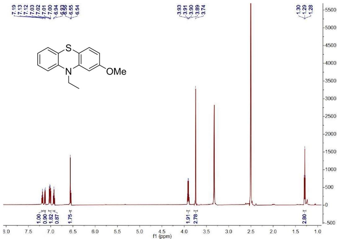
The <sup>1</sup>H NMR (600 MHz) spectra of **Compound 1** in DMSO-*d*<sub>6</sub>.
