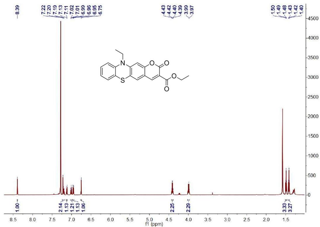
The  $^1\text{H}$  MNR (600 MHz) spectra of **Compound 4** in  $\text{CDCl}_3$ .
