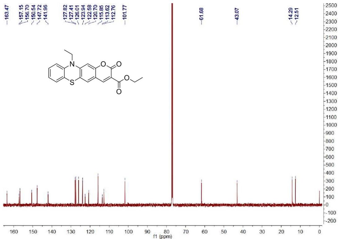
The  $^{13}\text{C}$  NMR (151 MHz) spectra of **Compound 4** in  $\text{CDCl}_3$ .
