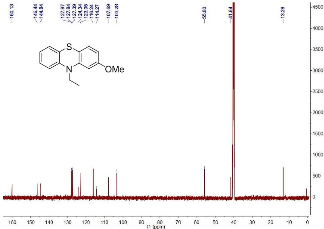
The <sup>13</sup>C NMR (151 MHz) spectra of **Compound 1** in DMSO-*d*<sub>6</sub>.
