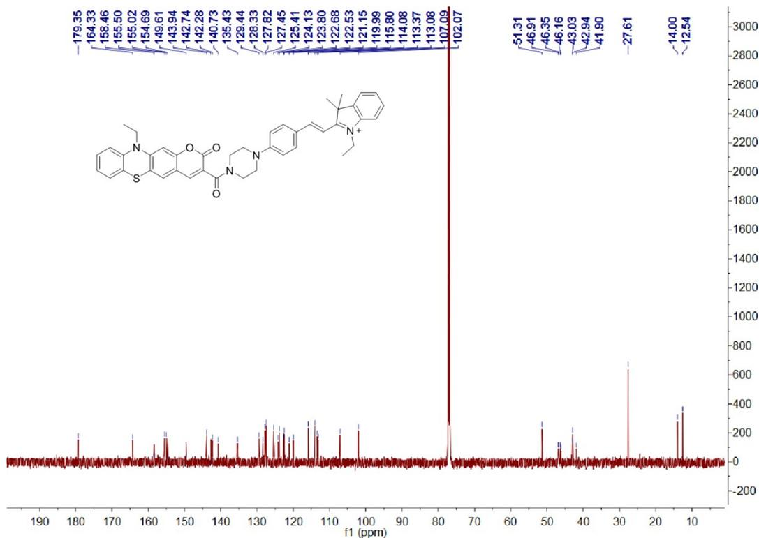
The  $^{13}\text{C}$  NMR (151 MHz) spectra of probe *PC* in  $\text{CDCl}_3$ .
