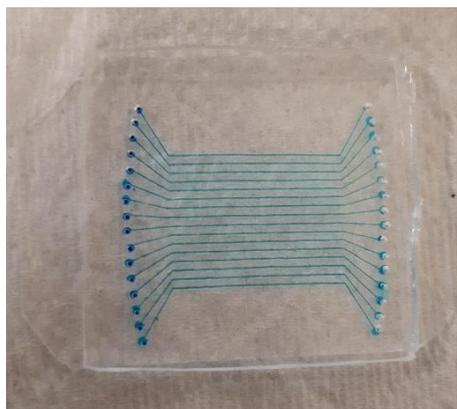
Figure S1: The microfluidic PDMS-glass chip with the PDMS slab sealed on a glass slide (50 mm × 75 mm) and filled with blue dyed solution for illustration.
