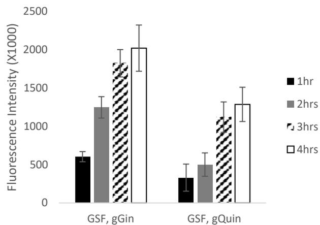
Figure S6: Optimization of LIDA reaction time for TF ligase. Signal intensities obtained in LIDA from different reaction times for GSF-containing lanes with either gGin or gQuin template. The ligation reactions contain Gin-NH<sub>2</sub> (10 nM), GSF (30  $\mu$ M), Det (25  $\mu$ M), Frag (25  $\mu$ M), MgCl<sub>2</sub> (20 mM) and 1.25 U/ $\mu$ L TF ligase.
