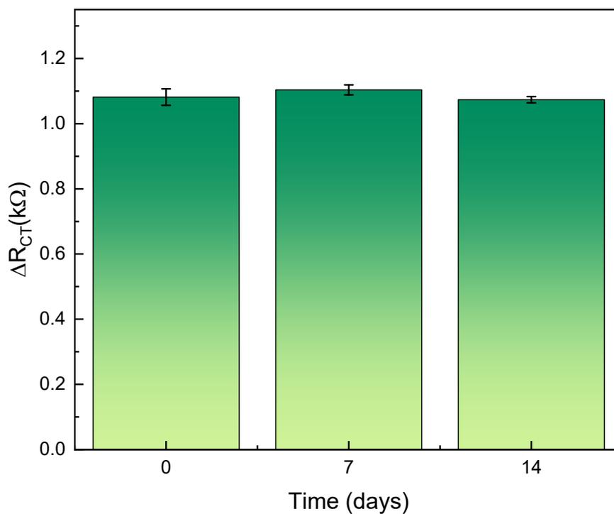
**Figure S5.** Stability of MIP sensors stored for different time
