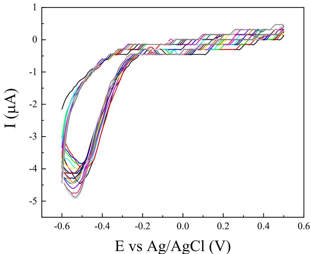
**Figure S1.** A cyclic voltammograms of AuNPs electrodeposition on SPCE
