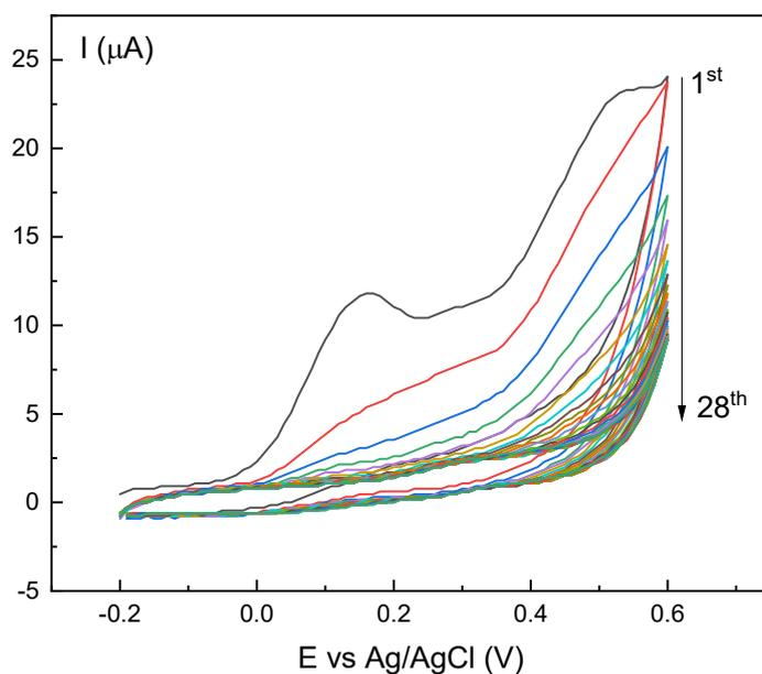
**Figure S3.** Cyclic voltammograms during the ENRO-MIP electro-polymerization on the AuNPs/SPCE at a scan rate of 50 mV/s.
