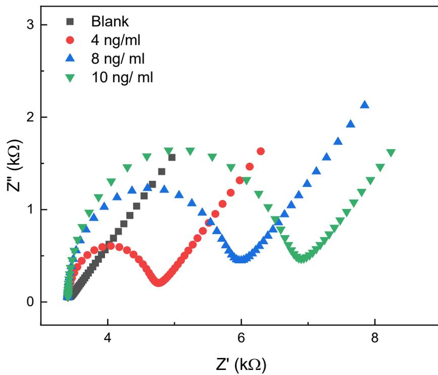
**Figure S6.** The Nyquist plots of impedance spectra corresponding to the response of ENRO-MIP sensor when exposing to aquaculture water samples containing different concentrations.
