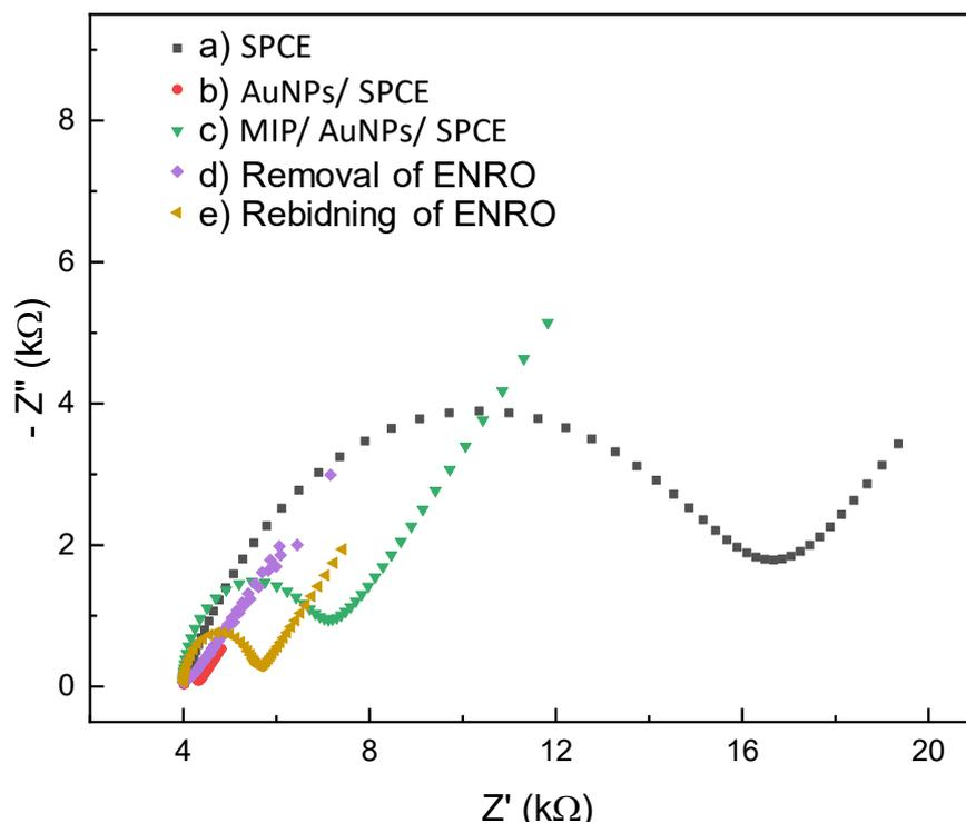
**Figure S4.** The Nyquist plots of impedance spectra corresponding to modification steps of SPCE for the development of the MIP sensor: a) bare SPCE; b) AuNPs/SPCE; c) ENRO-imprinted MIP/AuNPs/SPCE; d) ENRO-removal MIP/AuNPs/SPCE and rebinding of ENRO (at concentration of 5 ng/mL).
