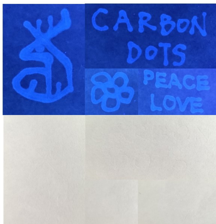
Fig. S4 Photographs of the fluorescent patterns hand-drawn by Y-CDs as the fluorescent inks under UV light (up) and daylight (down). The bright blue fluorescent patterns were observed in filter paper under UV light excitation, while the patterned filter paper seemed no apparent change under daylight, indicating its great application potential in anti-counterfeiting, information encryption and storage.
