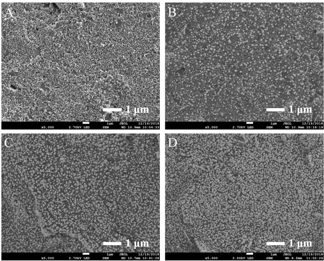
47 **Fig S5** The SEM images of the electrode surfaces with different electrodeposition times,
