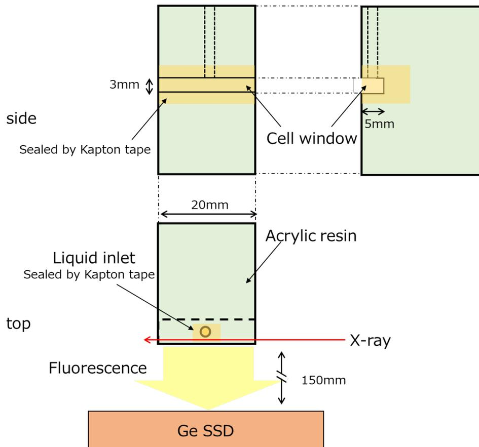
Figure S1. Experimental cell for X-ray absorption spectroscopy.
