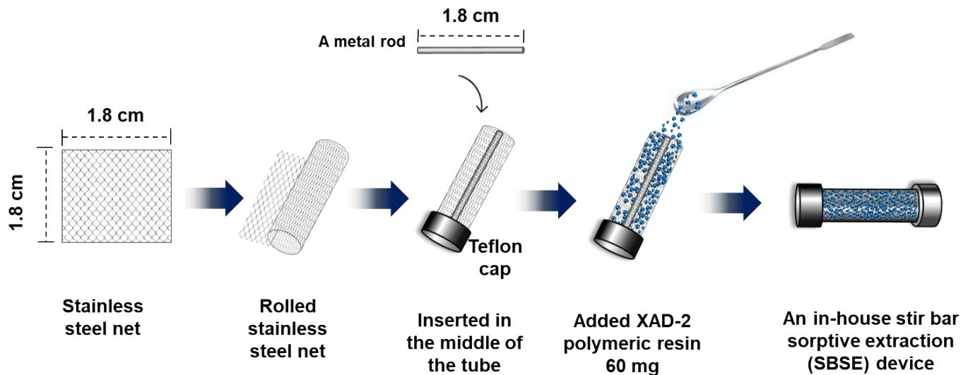
**Fig. S1** A schematic diagram representative an in-house SBSE device.
