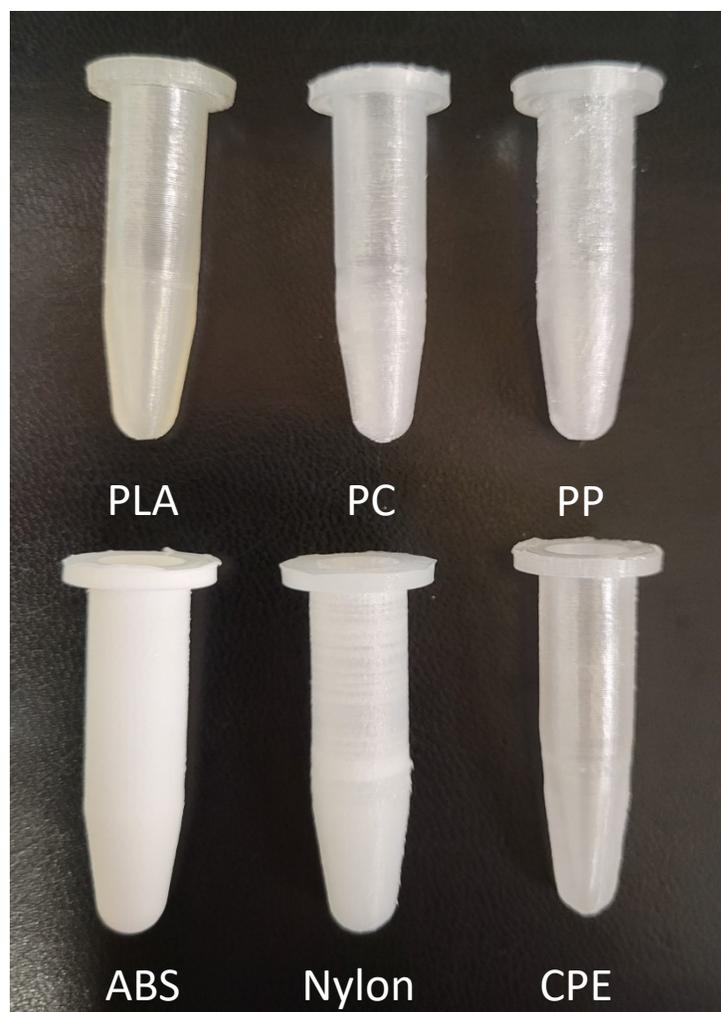
Figure S2. Images of 3D printed DNA storage devices used in the study. The thermoplastic filaments featured in the image are: polylactic acid (PLA), polycarbonate (PC), polypropylene (PP), acrylonitrile butadiene styrene (ABS), nylon, and co-polyester (CPE).
