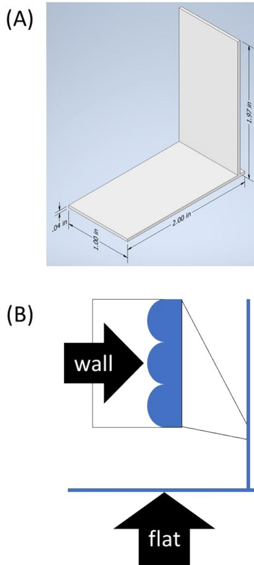
Figure S1. Schematic of 3D model designed for sessile drop contact angle measurements. Image (A) shows the 3D model featuring dimensions from Inventor software and (B) describes the expected surface morphologies following printing that were probed by contact angle measurements.
