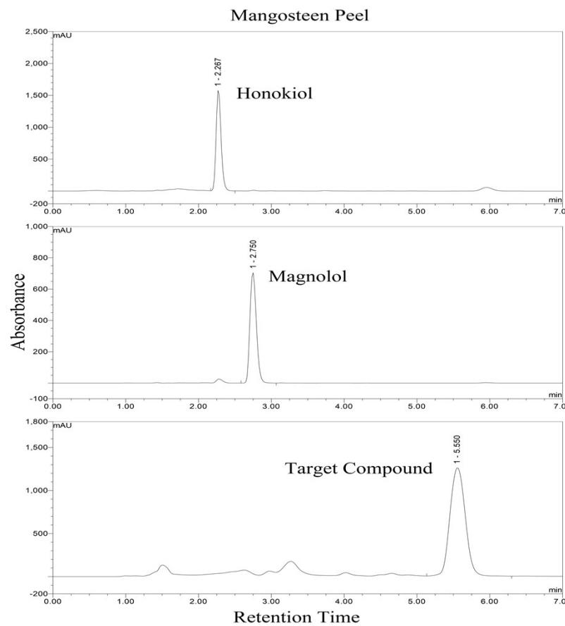
**Figure S3.** The HPLC chromatogram of mangosteen peel. Experimental conditions: column: Kromasil 100-5-C18 column (5  $\mu\text{m}$  particle size, 4.6  $\times$  150 mm); mobile phase: 90% methanol; column temperature: 30°C; detector temperature: 30°C; detection wavelength: 254 nm.
