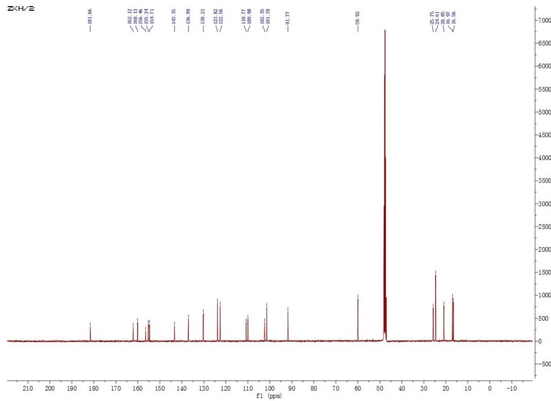
**Figure S8.**  $^{13}\text{C}$ -NMR (100 MHz,  $\text{CDCl}_3$ ) Spectrum of Compound 1.
