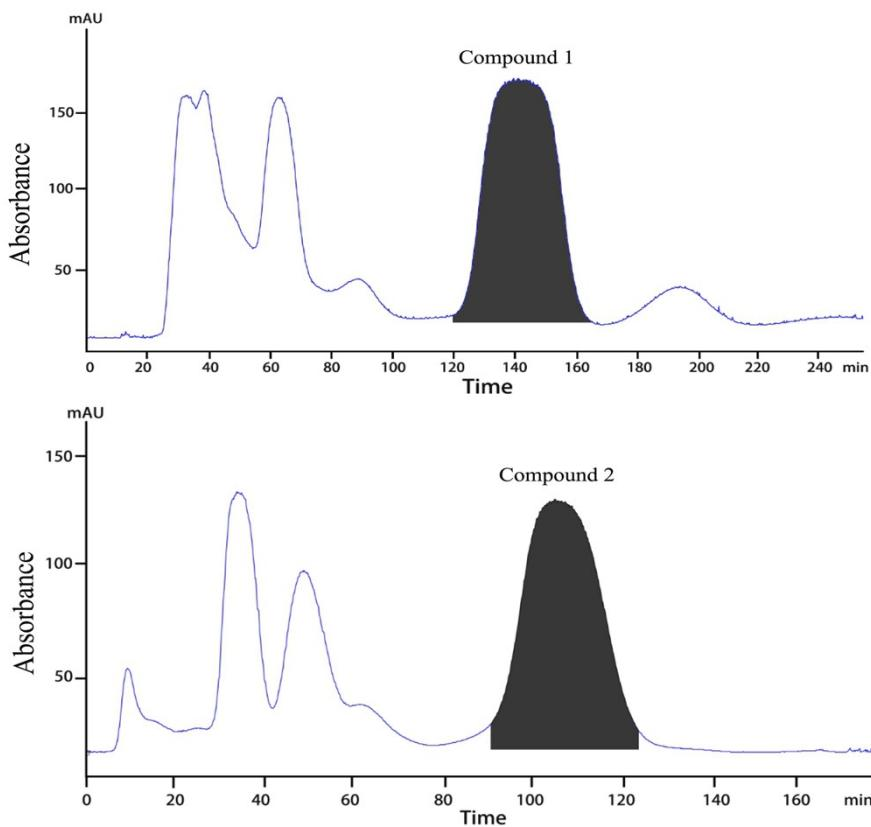
**Figure S5.** The HSCCC chromatogram of mangosteen peel and *H. sampsonii* Hance. Experimental conditions: solvent system: n-hexane-ethyl acetate-methanol-water (6:3:2:1 for mangosteen peel and 1:4:1:4 for *H. sampsonii* Hance, v/v/v/v); resolution speed: 900 rpm; separation temperature: 30°C; detection wavelength: 254 nm. The peaks marked in two chromatogram are mangostin and quercitrin.
