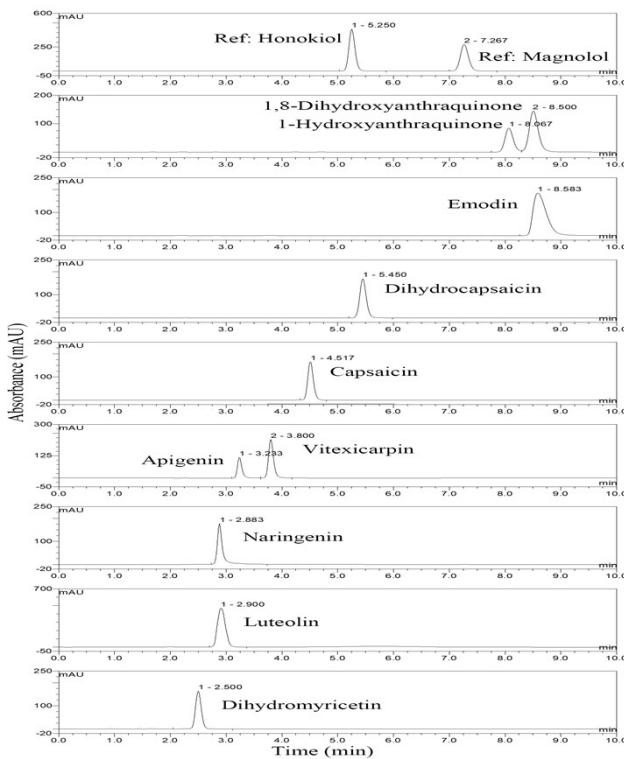
**Figure S2.** Representative HPLC chromatograms. Experimental conditions: column: Agilent ZORBAX SB-C18 column (5  $\mu$ m particle size, 4.6  $\times$  250 mm, marked as column 1); mobile phase: 80% methanol; flow rate: 1.0 mL/min; column temperature: 30°C; detector temperature: 30°C; detection wavelength: 254 nm.
