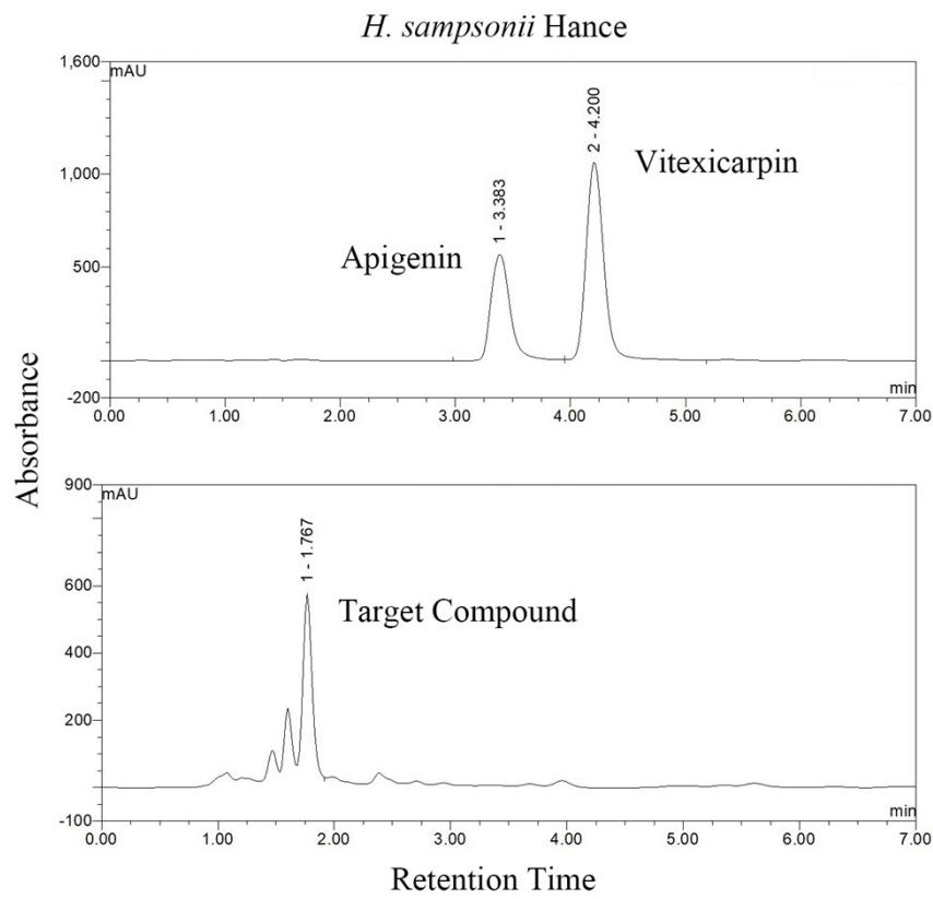
**Figure S4.** The HPLC chromatogram of *H. sampsonii* Hance. Experimental conditions: column: Agilent Eclipse XDB-C18 column (5  $\mu$ m particle size, 9.4  $\times$  250 mm); mobile phase: 60% methanol; column temperature: 30°C; detector temperature: 30°C; detection wavelength: 254 nm.
