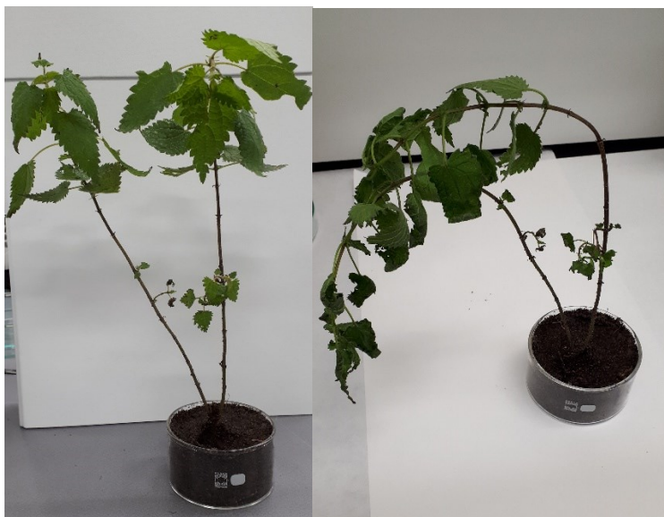
Figure A. 4. Nettle A) prior to exposure B) after 250 mg/m 3 exposure to sarin. It should be noted that the change could also be due to the dry atmosphere in the vapor generation set-up instead as a result of the chemical warfare agent exposure.
