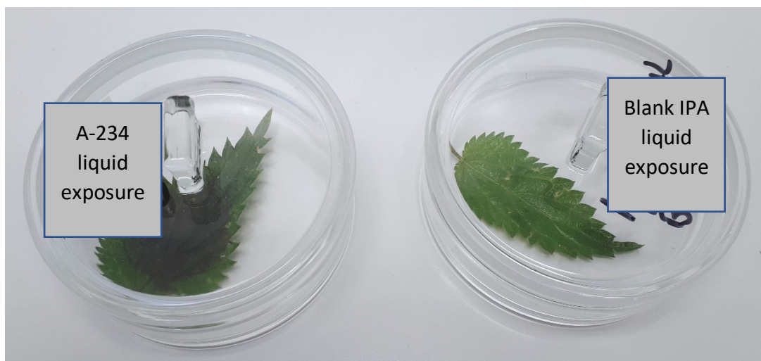
Figure A. 2. Physical state of nettle leaf upon liquid exposure to A-234.
