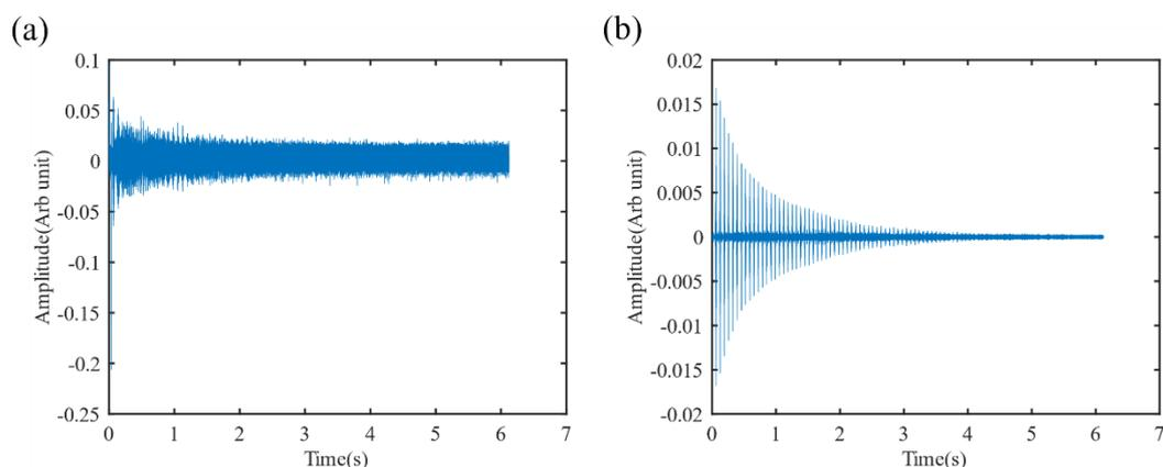
**Figure S1 (a).** The raw signal in time domain which was the image current induced by cytochrome C (16+) ions at  $1 \times 10^{-10}$  Torr with nitrogen as the buffer gas. **(b).** The raw signal filtered by a bandpass filter with passband of 186-187 kHz.
