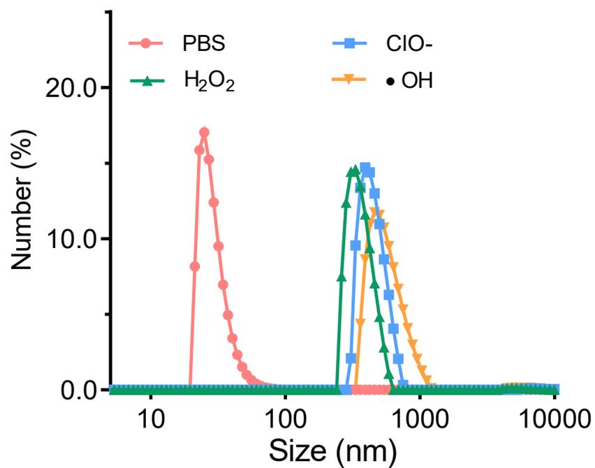
**Figure S17.** Size changes of SIP<sub>DOX</sub> in the presence of various ROS (H<sub>2</sub>O<sub>2</sub>: 10 mM, ClO<sup>-</sup>: 5 nM, •OH: 3.3 mM).
