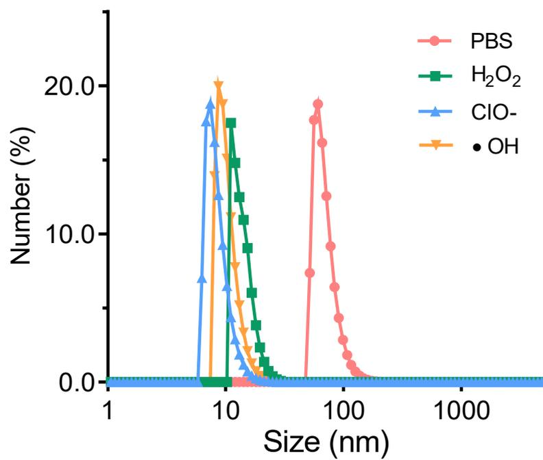
**Figure S19.** Size changes of TA<sub>CA</sub> in the presence of various ROS (H<sub>2</sub>O<sub>2</sub>: 10 mM, ClO<sup>-</sup>: 5 nM, •OH: 3.3 mM).
