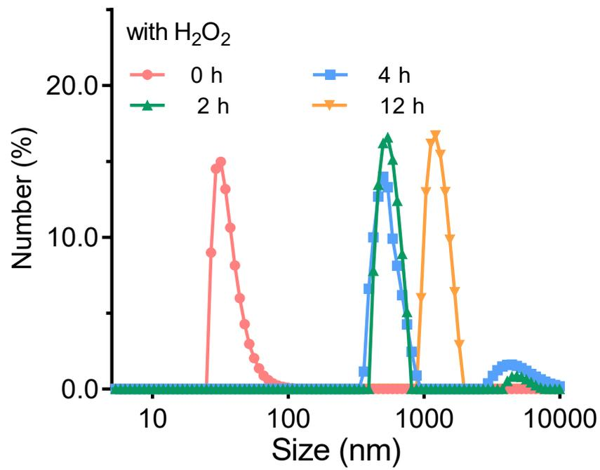
**Figure S16.** Size changes of SIP<sub>D0X</sub> after the addition of H<sub>2</sub>O<sub>2</sub> (10 mM) in PBS for different time.
