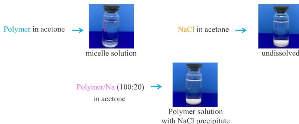
**Figure S4.** Dissolution of Polymer, NaCl and Polymer/Na in acetone.
