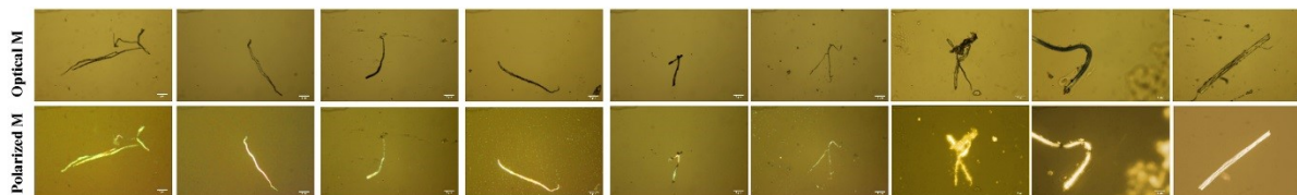
Figure S9: Nanotape or nanoribbon- like crystals seen at 37°C and pH 2 or 4 seen after 7 days.
