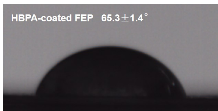
Fig. S5 Static water contact angle of HBPA-coated FEP.
