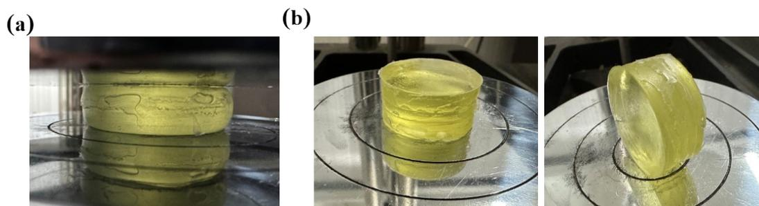
Fig. S3 The digital photographs of the specimen during (a) and after (b) 100 cycles of compressive testing.
