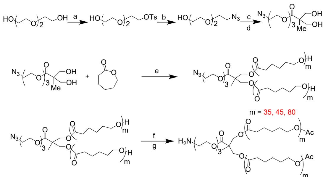
**Reagents:** (a) p-TsCl, dry TEA, dry DCM; (b) NaN<sub>3</sub>, DMF, refluxed at 100 °C; (c) Bis-MPA-acetonide, DCC, DPTS, dry DCM; (d) Amberlite Resin H<sup>+</sup>, MeOH, 40 °C; (e) Sn(oct)<sub>2</sub>, 85 °C; (f) dry DCM, dry TEA, CH<sub>3</sub>COCl; (g) Pd/C-H<sub>2</sub>, dry DCM.
