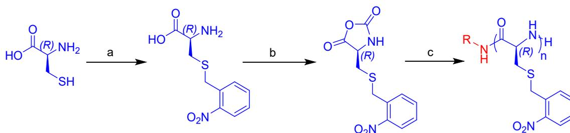
**Reagents:** (a) O-nitrobenzyl bromide, TEA, Water & MeOH; (b) Triphosgene, Dry THF, 55 °C; (c) R-NH<sub>2</sub>, DMF, Glove Box, 36 h.
