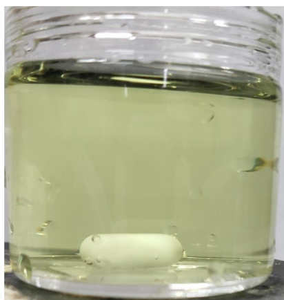
Fig. S6. 4-NP in pure water before (a) and after (b) adding \text{NaBH}_4 .
